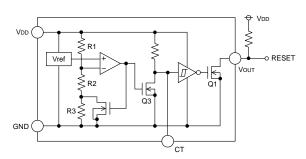
Fig.15 (BU42□□ type internal block diagram)
