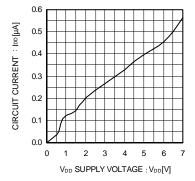
Fig.3 Circuit Current
