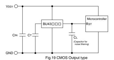
Application examples of BU42 == G/F/FVE series (Open Drain output type) and BU43 == G/F/FVE series (CMOS output type) are shown below.
