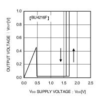
Fig.7 Operating Limit Voltage
