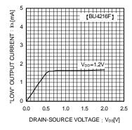
Fig.4 "LOW" Output Current
