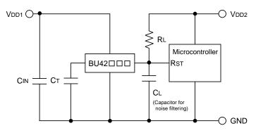
Fig.18 Open collector Output type
