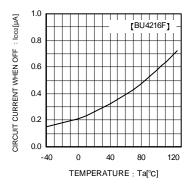
Fig.11 Circuit Current when OFF
