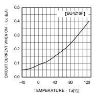
Fig.10 Circuit Current when ON
