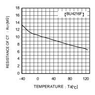
Fig.13 Ct Terminal Circuit Resistance
