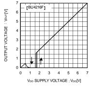
Fig.6 I/O Characteristics
