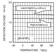
Fig.9 Detecting Voltage Release Voltage
