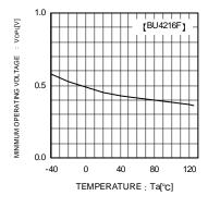
Fig.12 Operating Limit Voltage
