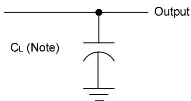
Note:  $C_L$  includes probe and jig capacitance.
