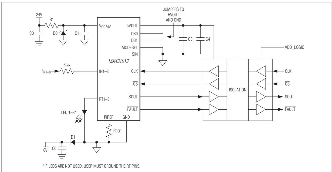
Figure 1. Typical EMC Protection Circuitry
