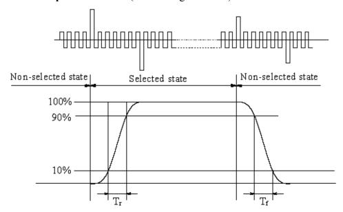
Turn on time:  $t_{on} = t_r$  Turn off time:  $t_{off} = t_f$
