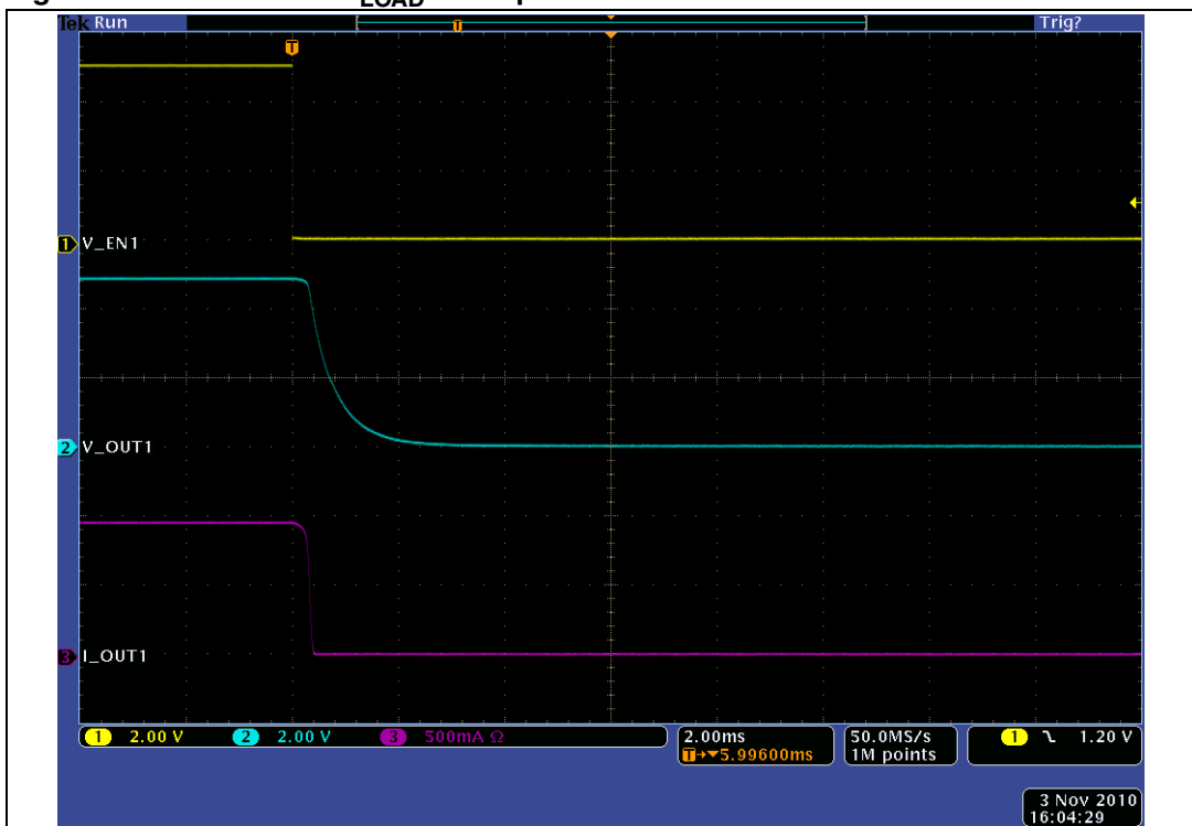
Figure 33. Turn-off for C_{LOAD} = 100 \mu F
