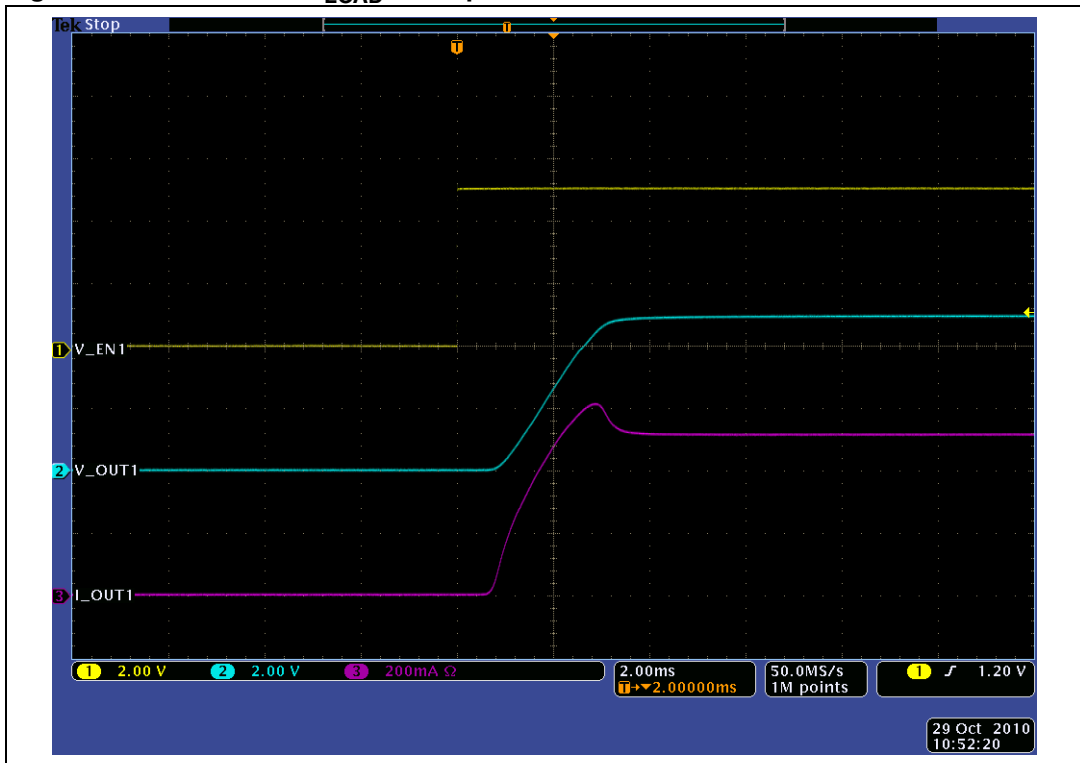
Figure 11. Turn-on for C_{LOAD} = 470 \mu F
