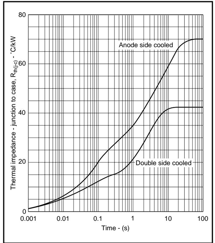
Fig.3 Transient thermal impedance - junction to case
