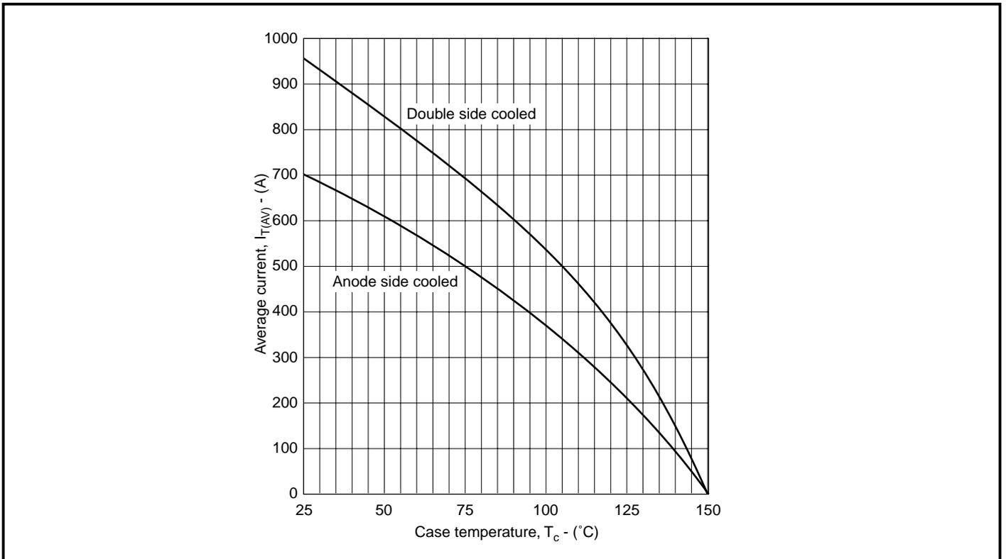
Fig.4 Average current rating vs temperature
