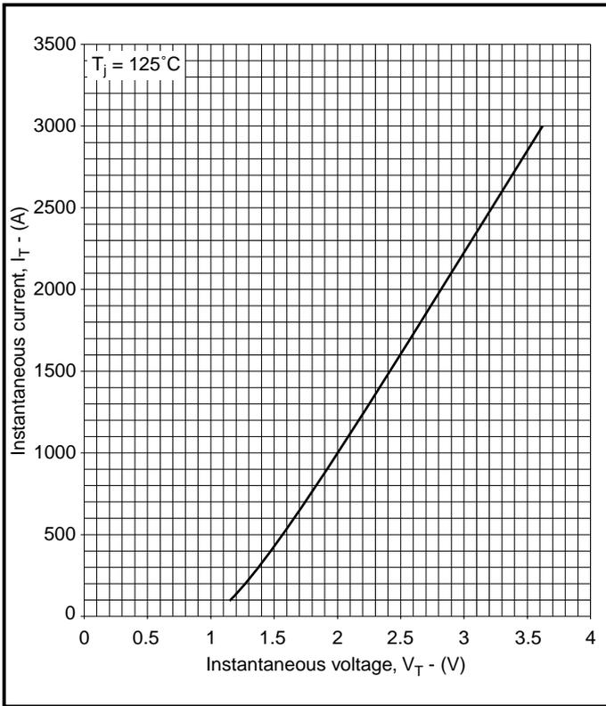
Fig.2 On-state characteristics
