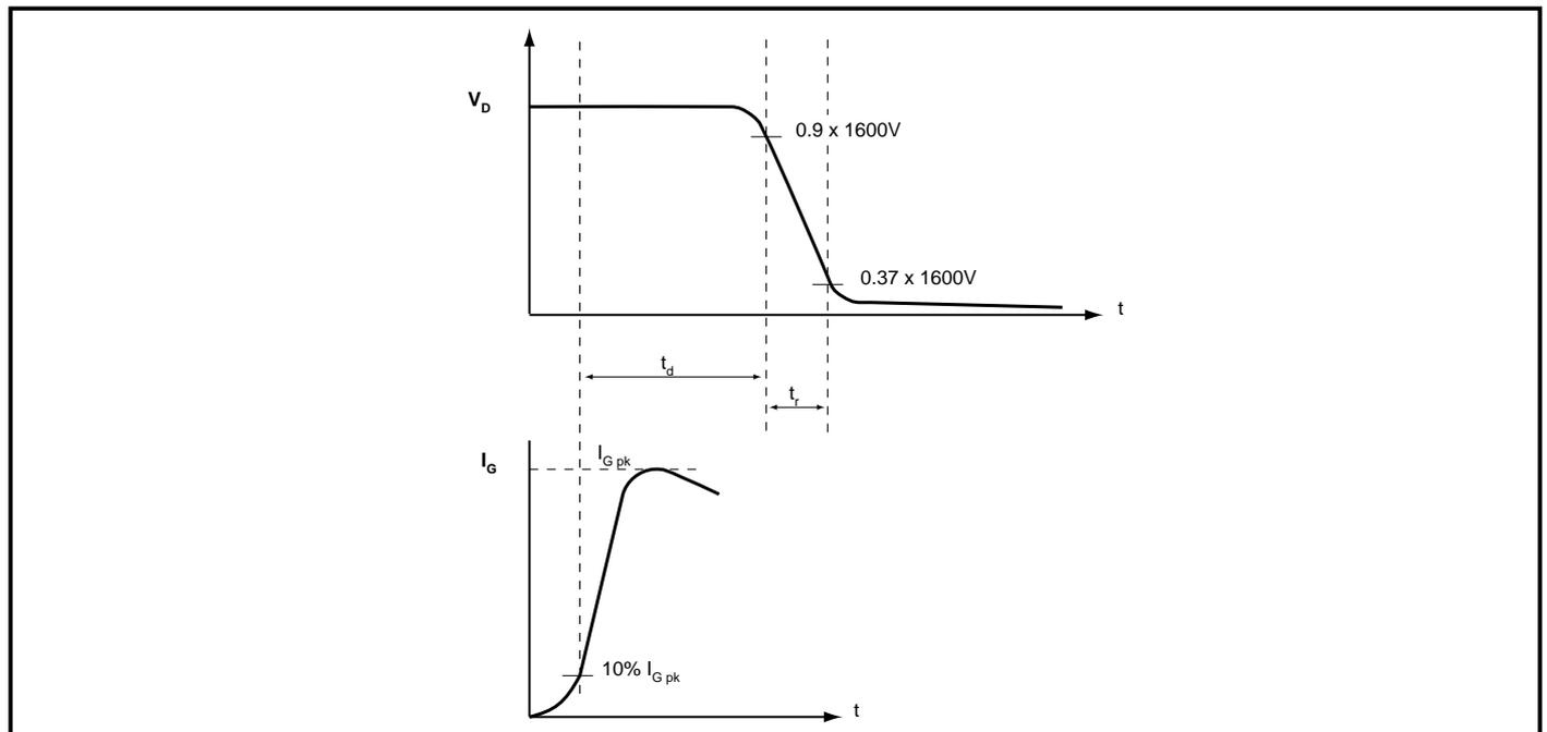
**Fig.1 Turn-on time measurement**
