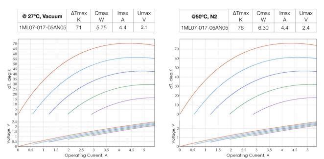
**Note**: Performance data is specified for optimal conditions (TEC hot side is stabilized at ambient temperature). Heatsink thermal resistance is not included into estimations. Use TECCad Software for estimations under different conditions.
