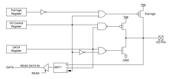
In SH69P48A, each output port contains a latch, which can hold the output data. Writing the port data register (PDR) under the output mode can directly transfer data to the corresponding pad.
