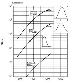
Typical Pulse Height Distributions for Two-and Three-Stage MCP
