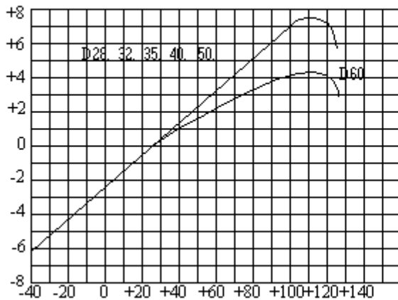
FIGURE 3-NORMALIZED VBO CHANGE VS JUNCTION TEMPERATURE
