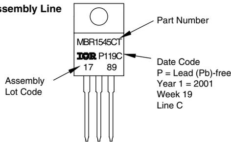
Example: This is a MBR1545CT with Assembly Lot Code 1789, assembled on WW 19, 2001 in the assembly line "C"
