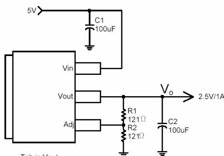
$$\text{Note: } V_o = V_{\text{REF}} * \left(1 + \frac{R_2}{R_1}\right)$$
