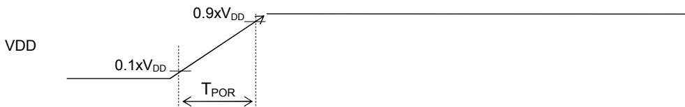
Power-on reset activation power rise time ( T_{POR} )
