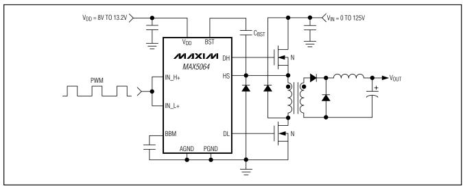
Figure 4. Two-Switch Forward Conversion
