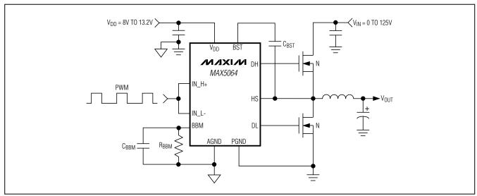
Figure 3. Synchronous Buck Converter
