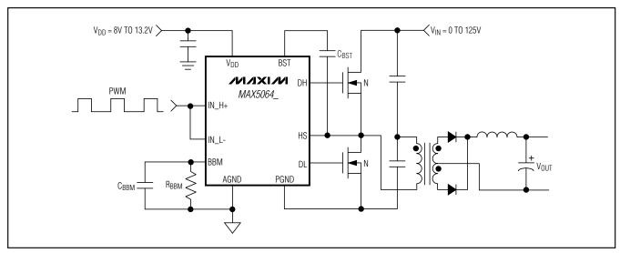
Figure 5. MAX5064 Half-Bridge Converter
