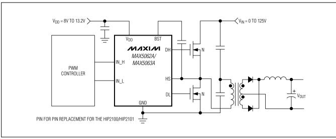
Figure 2. MAX5062 Half-Bridge Conversion
