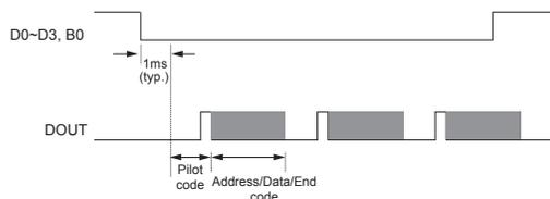
The transmission sequence is Pilot, Address, Data, End code.
