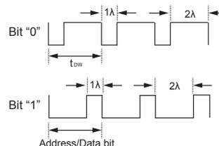
Note: 1. Bit "0" consists of a "low" pulse for  $1\lambda$  then changes to a "high" pulse for  $2\lambda$ .
