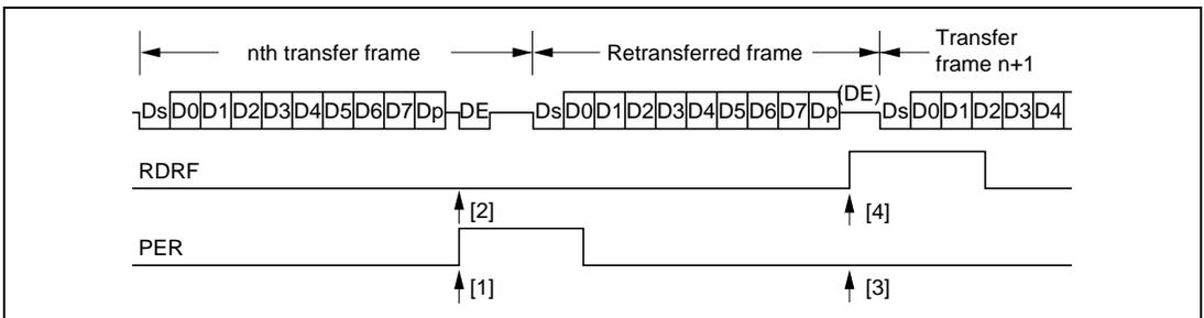
**Figure 13.11 Retransfer Operation in SCI Receive Mode**
