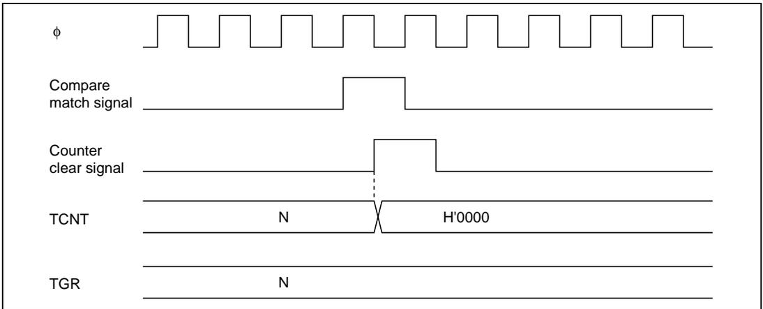
**Figure 9.34 Counter Clear Timing (Compare Match)**
