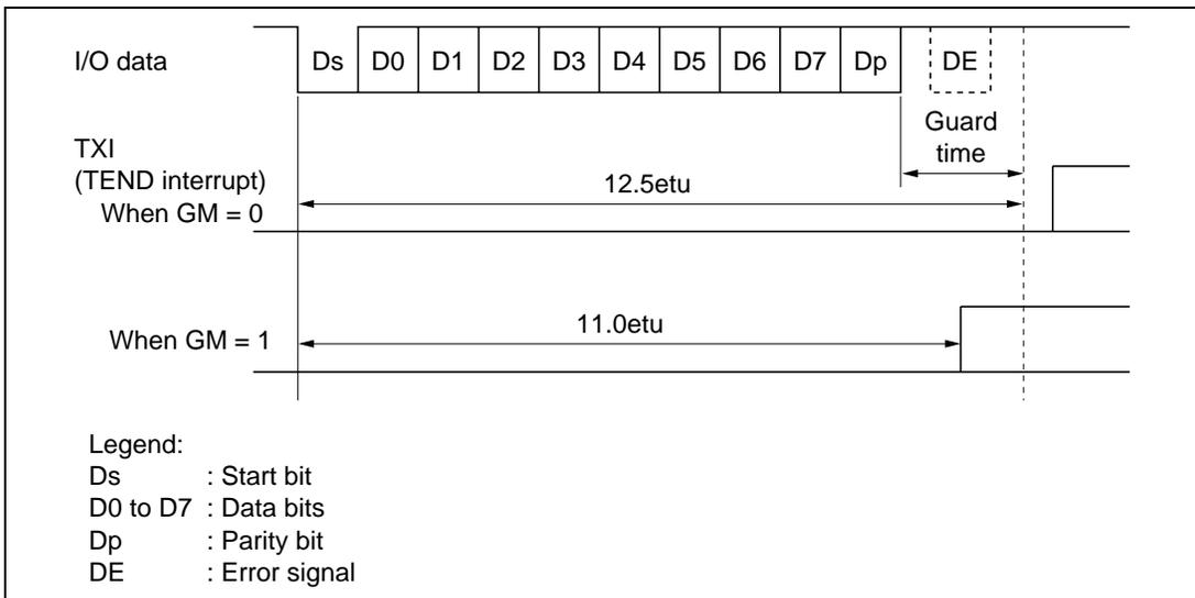
**Figure 13.6 TEND Flag Generation Timing in Transmission Operation**
