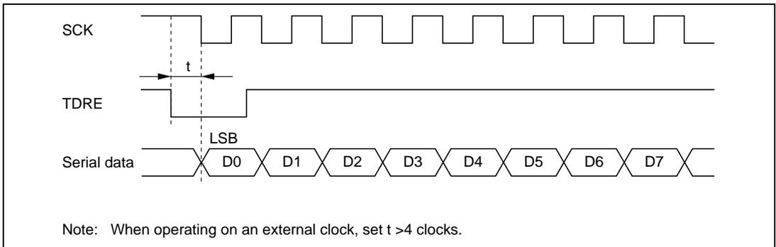
**Figure 12.22** Example of Clocked Synchronous Transmission by DTC
