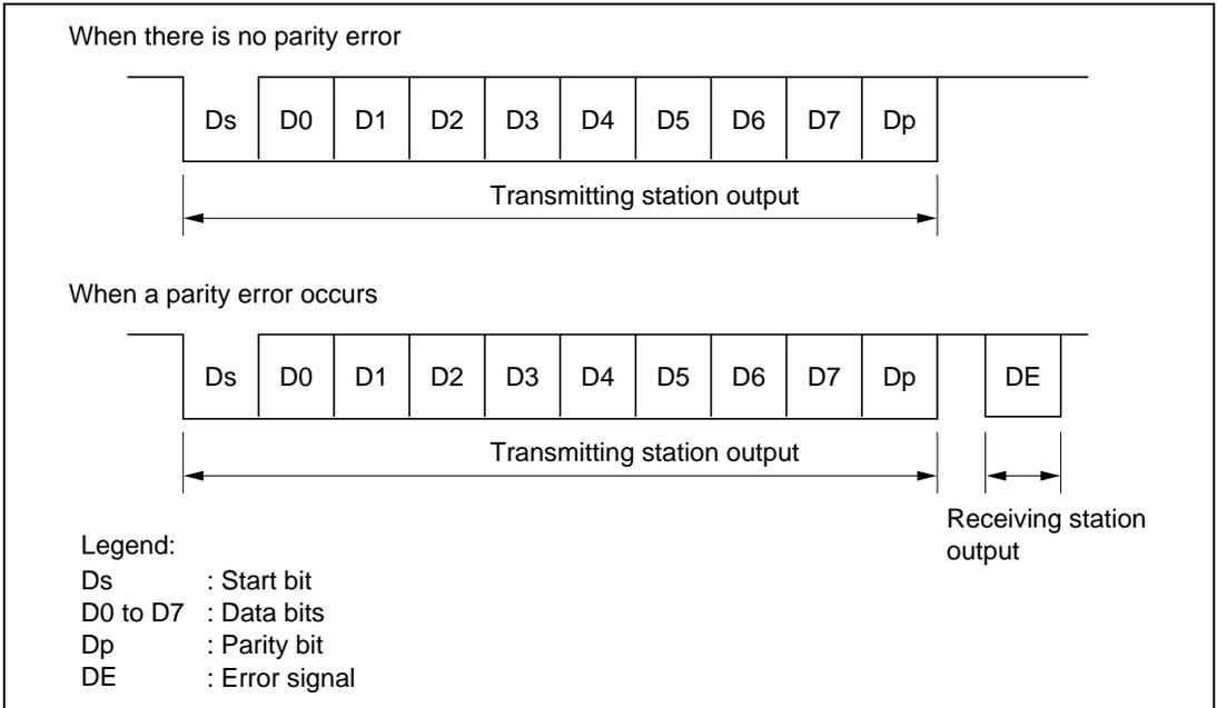
**Figure 13.3 Smart Card Interface Data Format**
