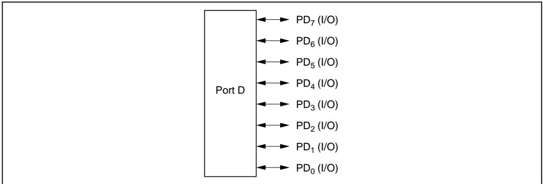
**Figure 8.20 Port D Pin Functions (Modes 3 and 7)**
