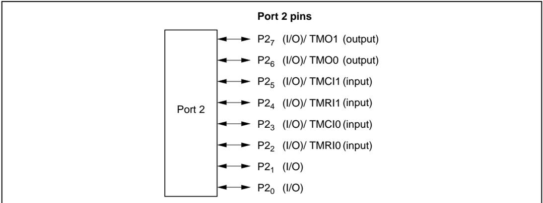
**Figure 8.2 Port 2 Pin Functions**
