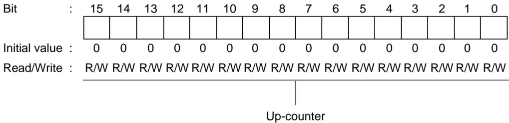
**TGR0A—Timer General Register 0A****H'FFD8****TPU0****TGR0B—Timer General Register 0B****H'FFDA****TPU0****TGR0C—Timer General Register 0C****H'FFDC****TPU0****TGR0D—Timer General Register 0D****H'FFDE****TPU0**
