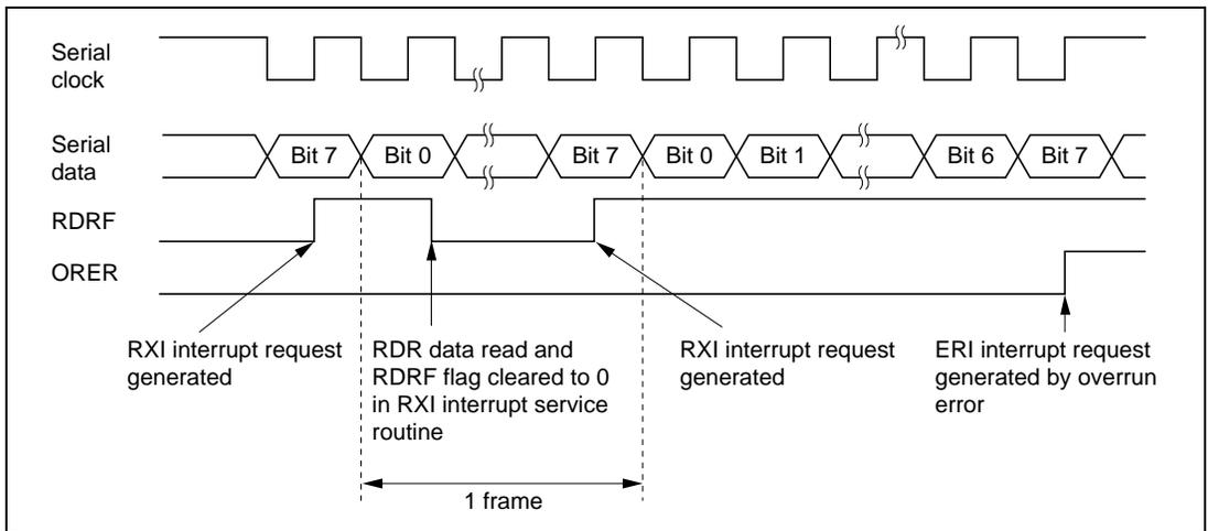
**Figure 12.19 Example of SCI Operation in Reception**
