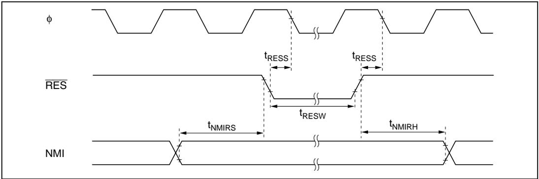
Figure 19.6 Reset Input Timing
