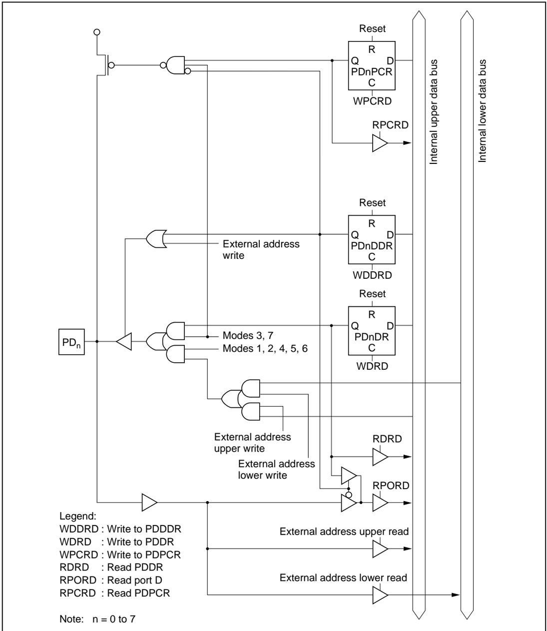
**Figure C.9 Port D Block Diagram (Pins PD<sub>0</sub> to PD<sub>7</sub>)**
