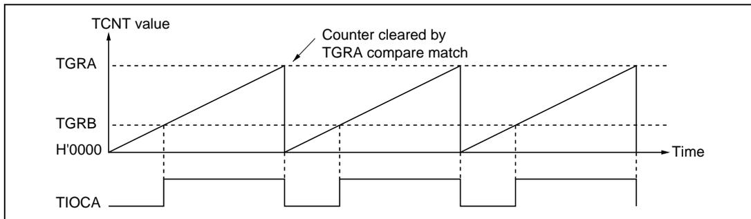
**Figure 9.22 Example of PWM Mode Operation (1)**
