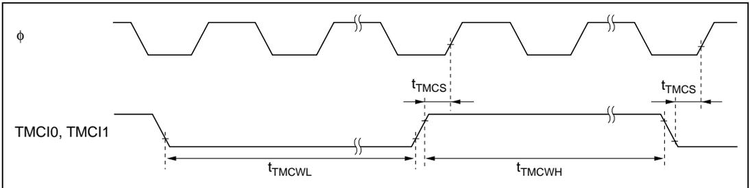
**Figure 19.19 8-Bit Timer Clock Input Timing**
