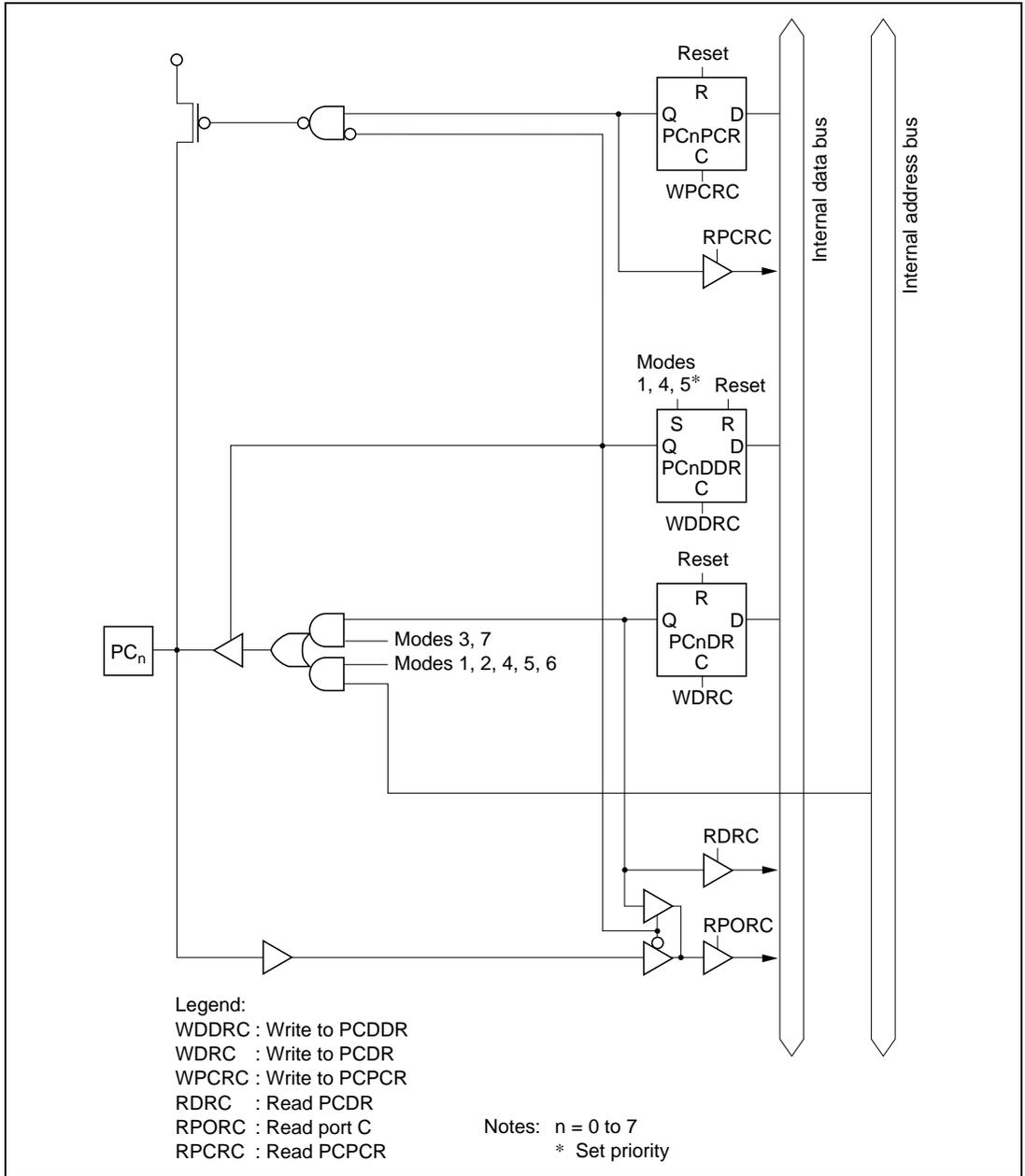
**Figure C.8 Port C Block Diagram (Pins PC<sub>0</sub> to PC<sub>7</sub>)**
