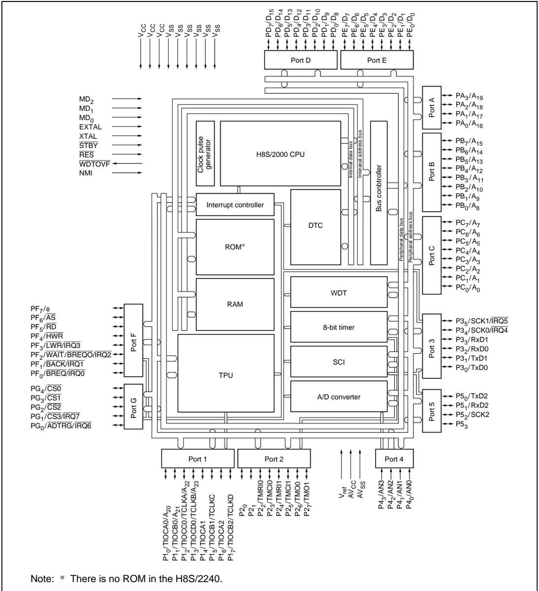
Figure 1.1 Block Diagram
