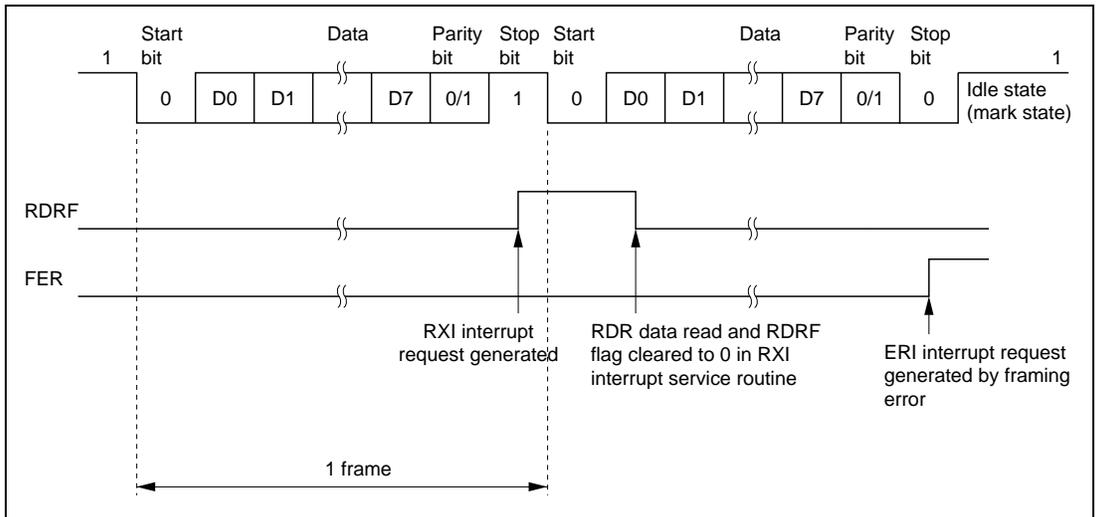
**Figure 12.8 Example of SCI Operation in Reception
