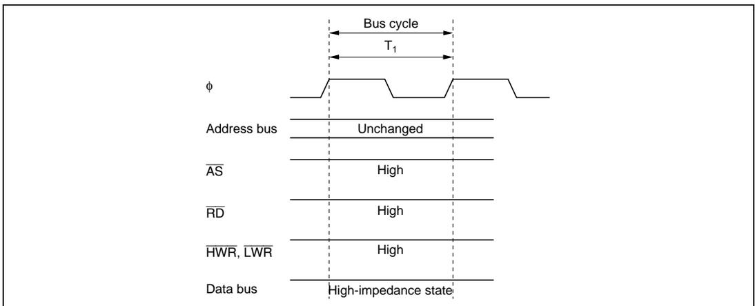
**Figure 6.5 Pin States during On-Chip Memory Access**
