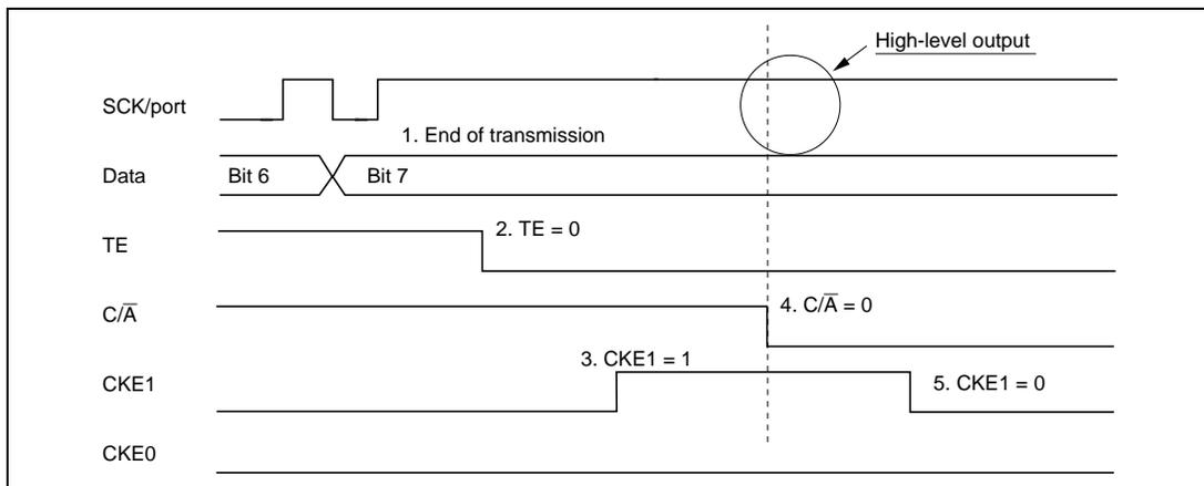
**Figure 12.28 Operation when Switching from SCK Pin Function to Port Pin Function
