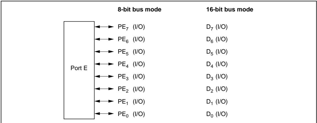
**Figure 8.22 Port E Pin Functions (Modes 1, 2, 4, 5, and 6)**
