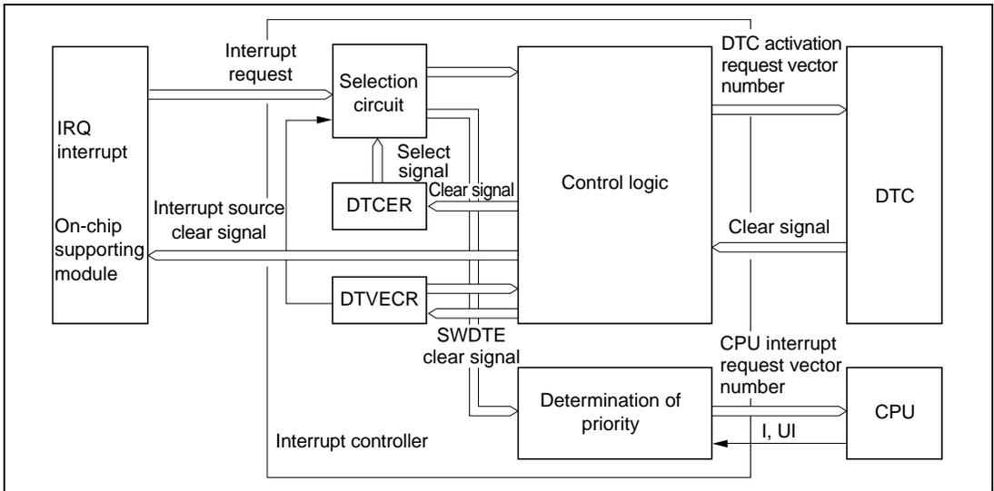
**Figure 5.10 Interrupt Control for DTC**
