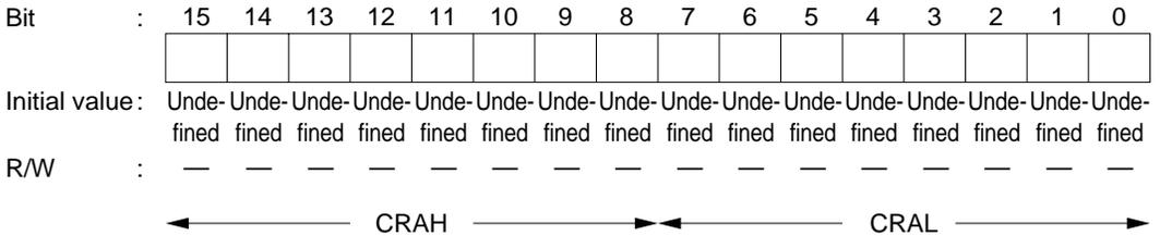
CRA is a 16-bit register that designates the number of times data is to be transferred by the DTC.
