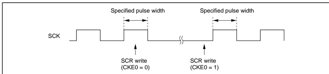
**Figure 13.8** Timing for Fixing Clock Output Level
