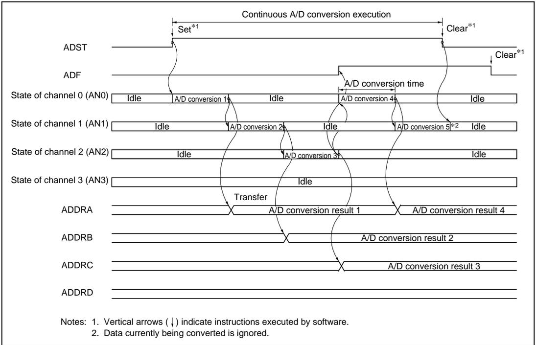
**Figure 14.4 Example of A/D Converter Operation
