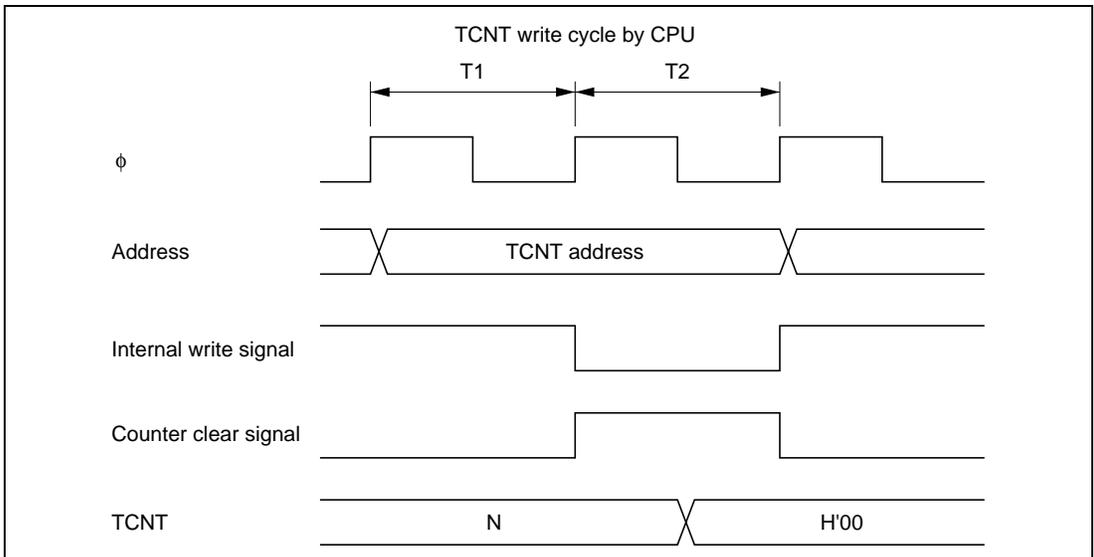
**Figure 10.10 Contention between TCNT Write and Clear**
