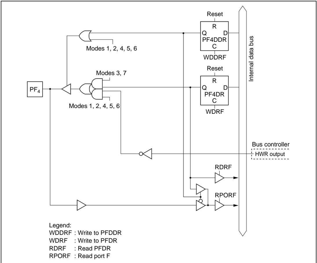
**Figure C.11 (e) Port F Block Diagram (Pin PF<sub>4</sub>)**
