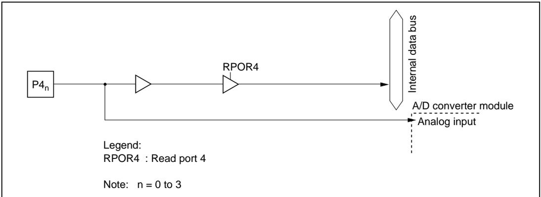
**Figure C.4 Port 4 Block Diagram (Pins  $P4_0$  to  $P4_3$ )**
