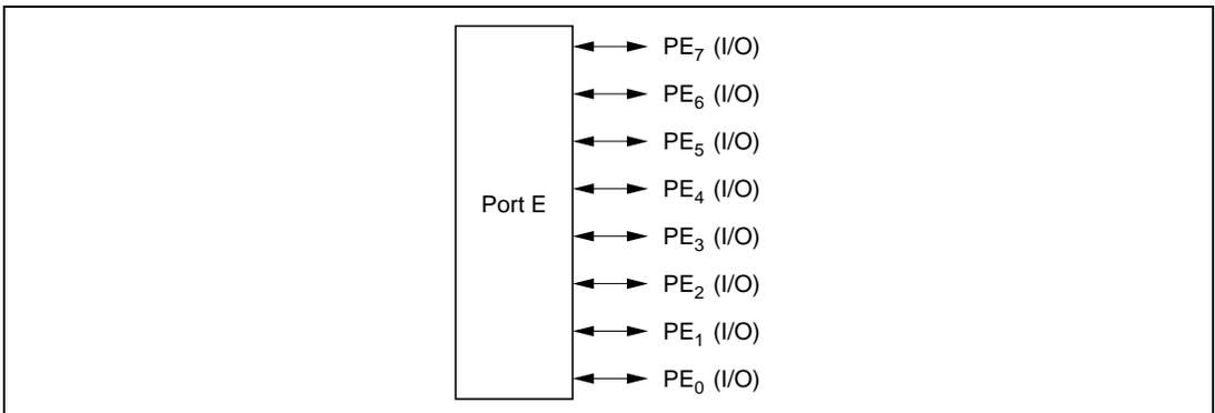
**Figure 8.23 Port E Pin Functions (Modes 3 and 7)**
