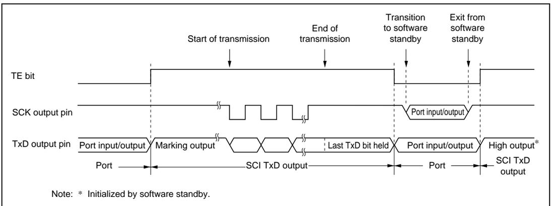
**Figure 12.25 Synchronous Transmission Using Internal Clock**
