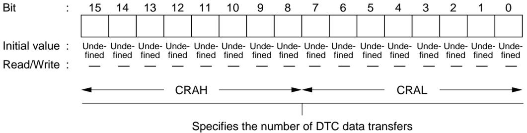
**CRB—DTC Transfer Count Register B****H'F800—H'FBFF****DTC**
