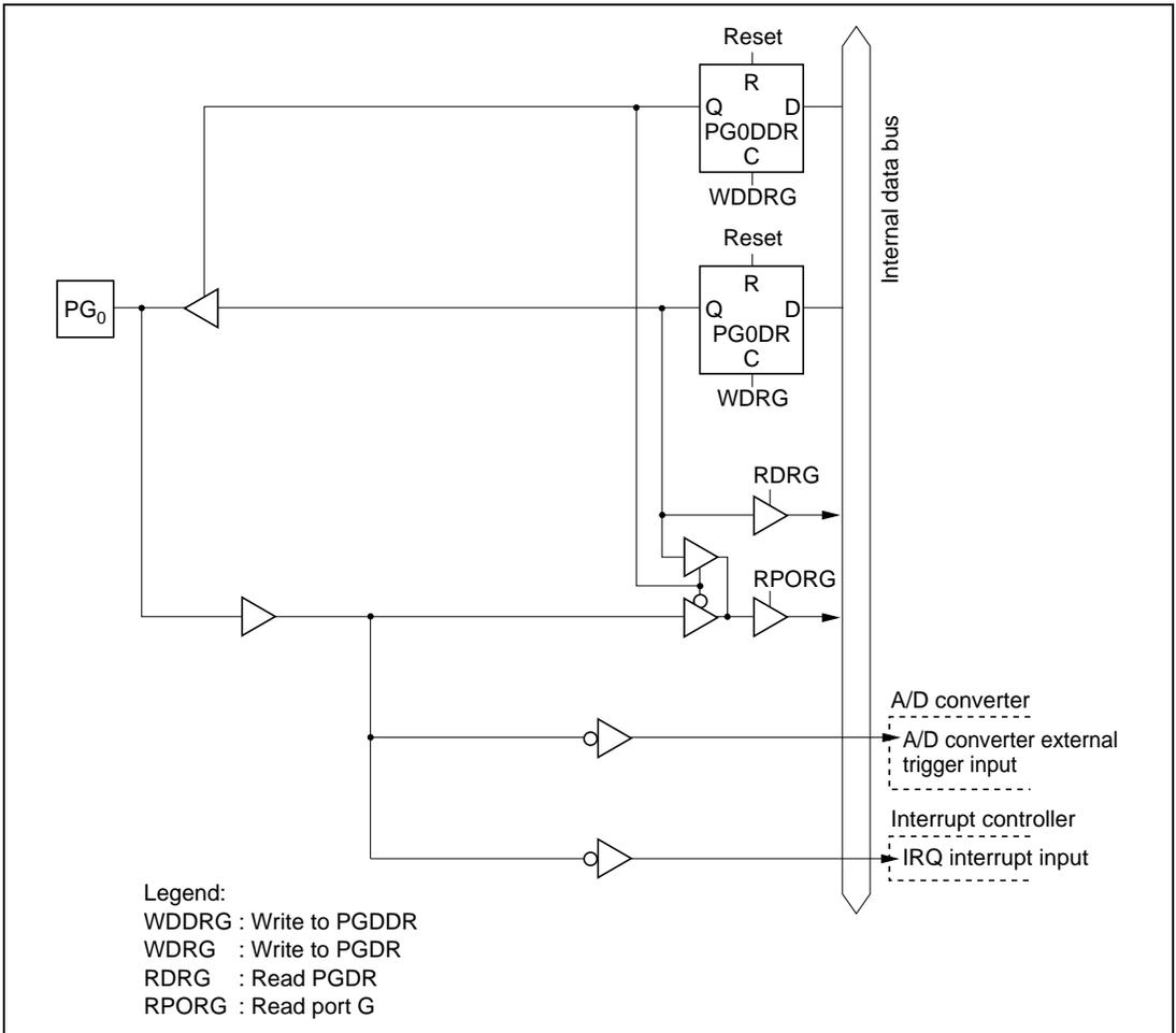
Figure C.12 (a) Port G Block Diagram (Pin  $PG_0$ )
