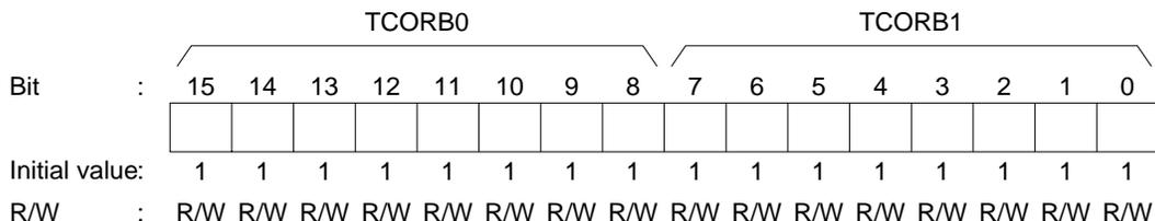
TCORB0 and TCORB1 are 8-bit readable/writable registers. TCORB0 and TCORB1 comprise a single 16-bit register so they can be accessed together by word transfer instruction.
