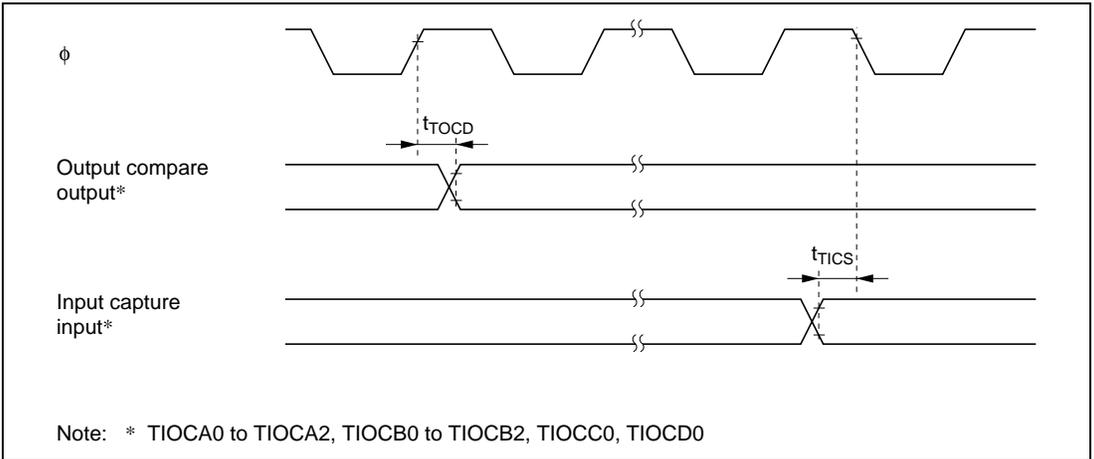
**Figure 19.16 TPU Input/Output Timing**
