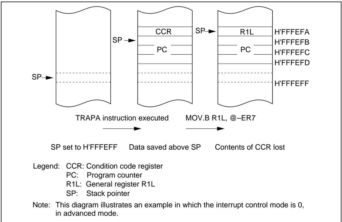
**Figure 4.6 Operation when SP Value is Odd**
