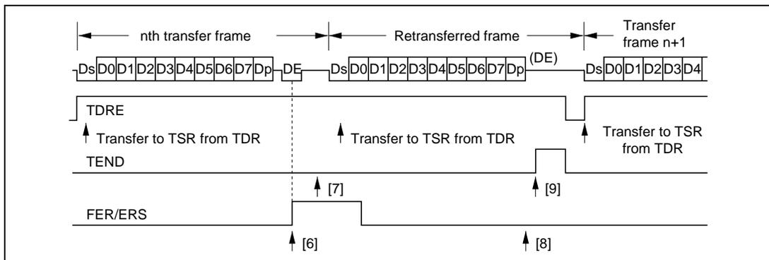
**Figure 13.12 Retransfer Operation in SCI Transmit Mode**
