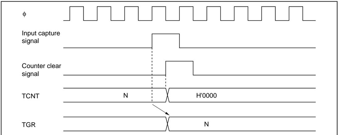
**Figure 9.35 Counter Clear Timing (Input Capture)**
