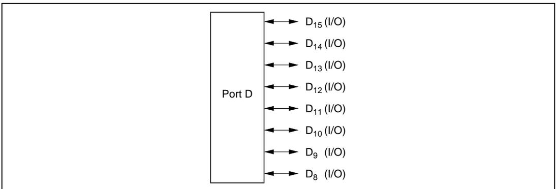
**Figure 8.19 Port D Pin Functions (Modes 1, 2, 4, 5, and 6)**
