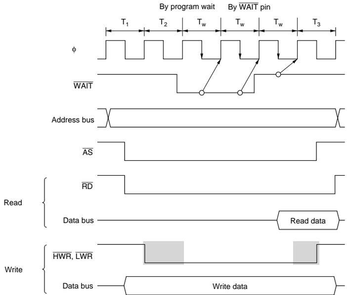
Note: / indicates the timing of  $\overline{\text{WAIT}}$  pin sampling.
