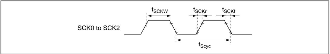
**Figure 19.22 SCK Clock Input Timing**
