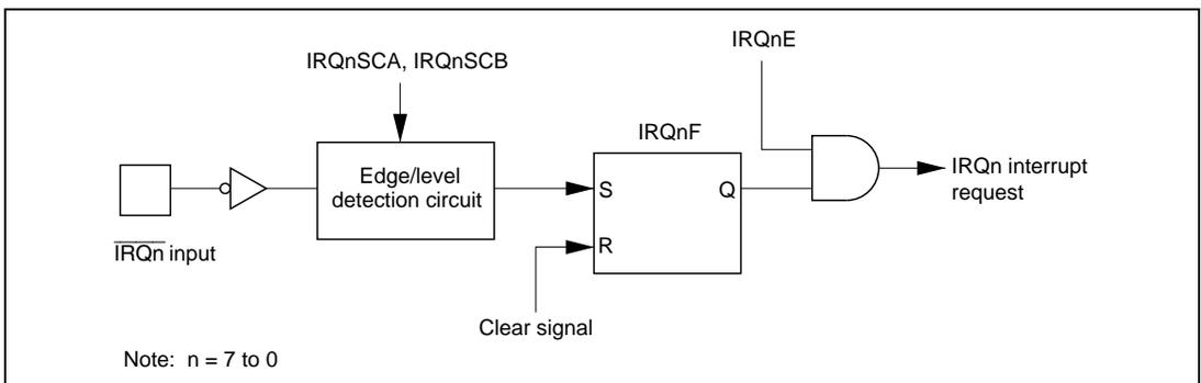
**Figure 5.2 Block Diagram of Interrupts IRQ7 to IRQ0**
