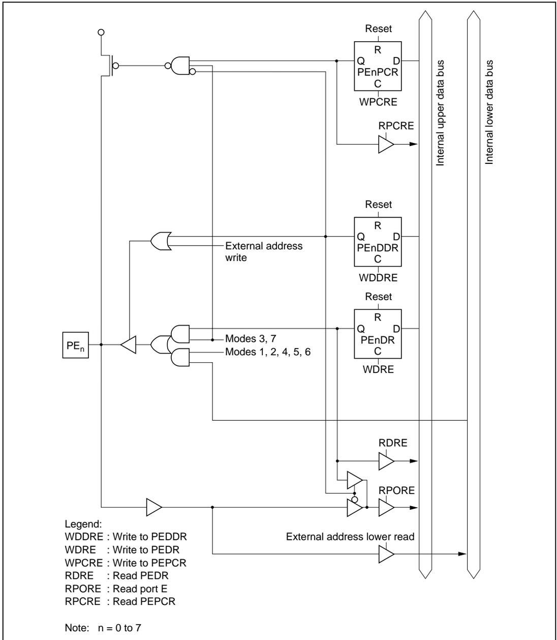
**Figure C.10 Port E Block Diagram (Pins PE<sub>0</sub> to PE<sub>7</sub>)**
