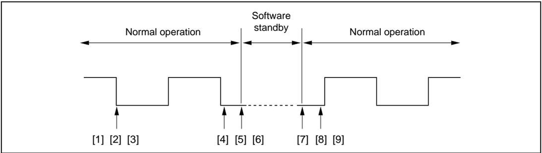
**Figure 13.9 Clock Halt and Restart Procedure**
