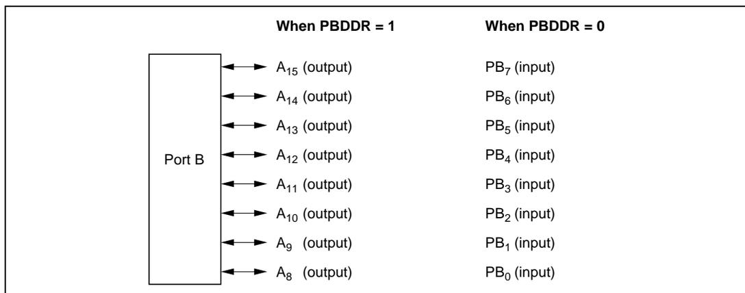
**Figure 8.12 Port B Pin Functions (Modes 2 and 6)**
