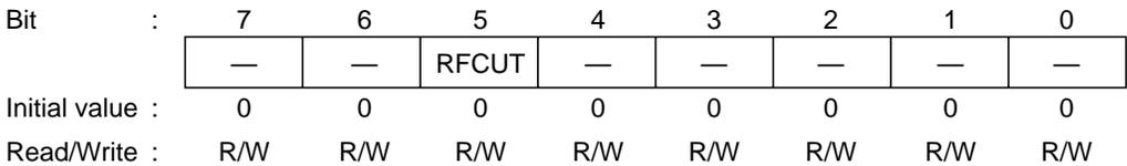
Control of Oscillator's Built-In Feedback Resistor in External Clock Input
