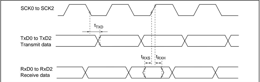
**Figure 19.23 SCI Input/Output Timing Synchronous Mode**
