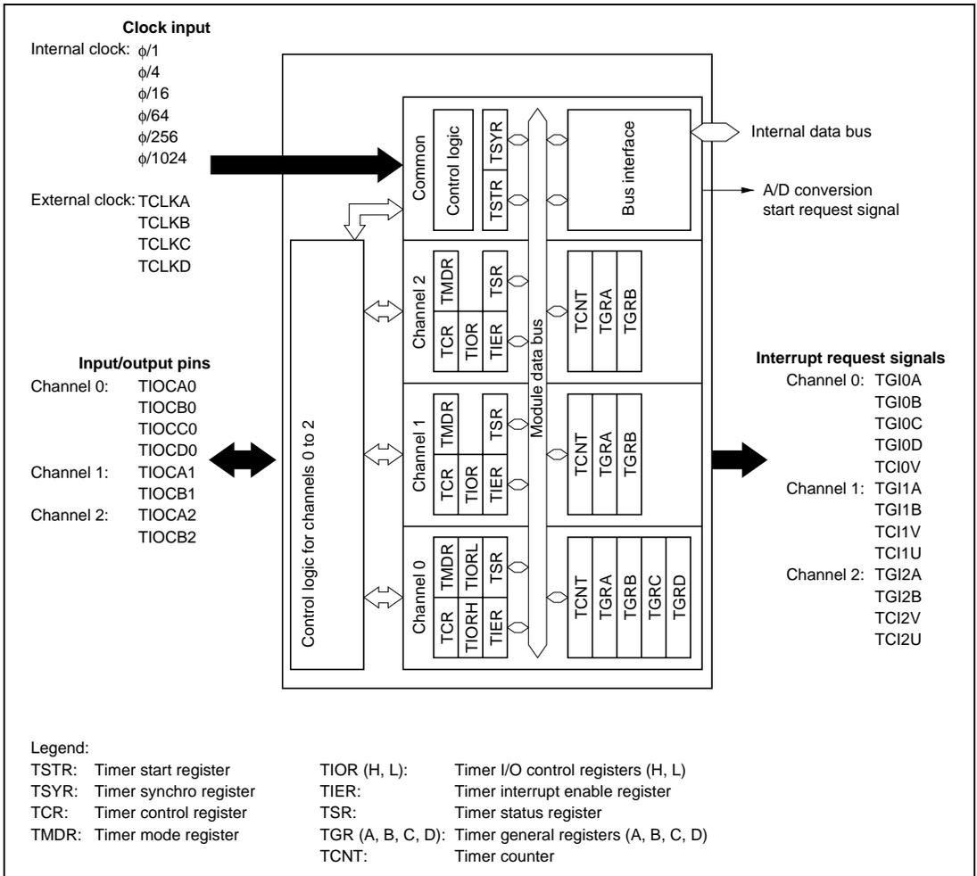
**Figure 9.1 Block Diagram of TPU**
