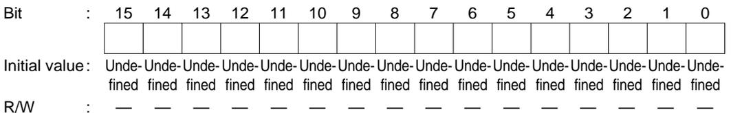
CRB is a 16-bit register that designates the number of times data is to be transferred by the DTC in block transfer mode. It functions as a 16-bit transfer counter (1 to 65536) that is decremented by 1 every time data is transferred, and transfer ends when the count reaches H'0000.
