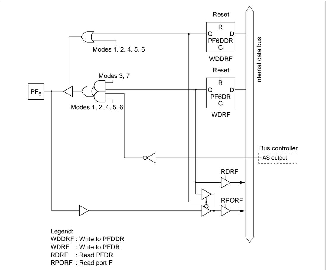
**Figure C.11 (g) Port F Block Diagram (Pin PF<sub>6</sub>)**
