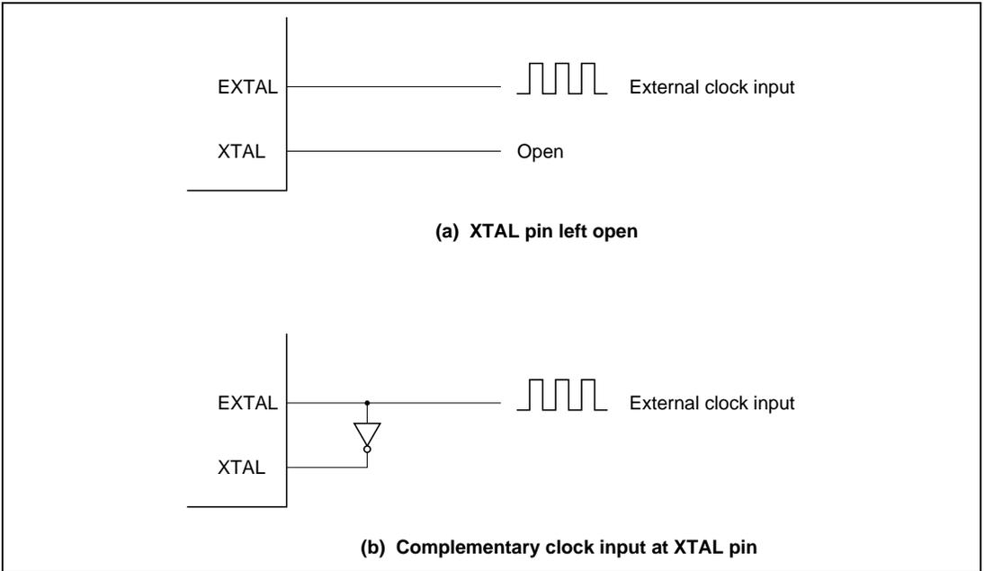
Figure 17.5 External Clock Input (Examples)
