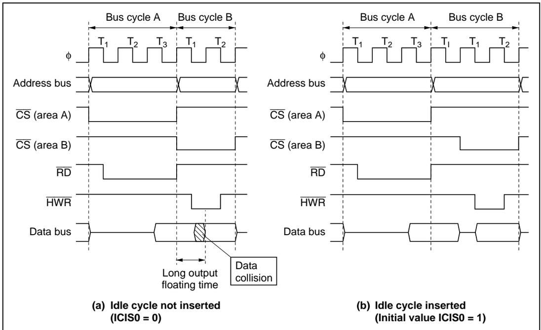
**Figure 6.21 Example of Idle Cycle Operation (2)**
