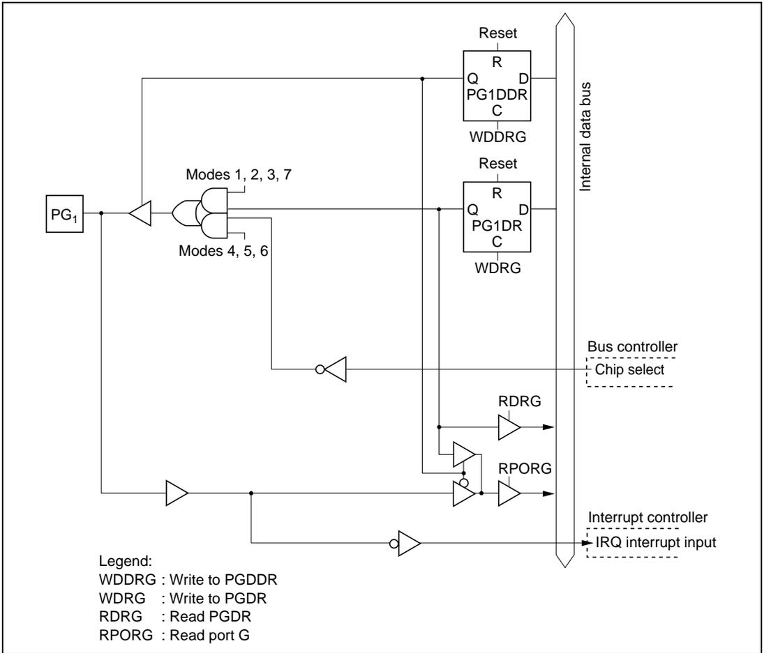
Figure C.12 (b) Port G Block Diagram (Pin PG<sub>1</sub>)
