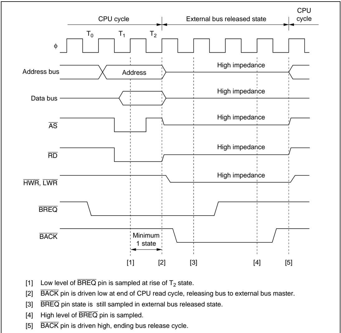
**Figure 6.23 Bus-Released State Transition Timing**
