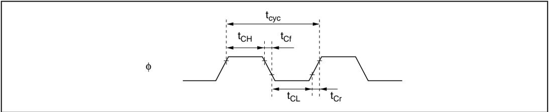
**Figure 19.4 System Clock Timing**
