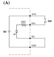
(A) Using Internal 5V auxiliary source
