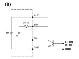
(B) ON/OFF Control by NPN transistor
