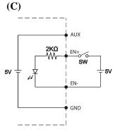
(C) Using external voltage source
