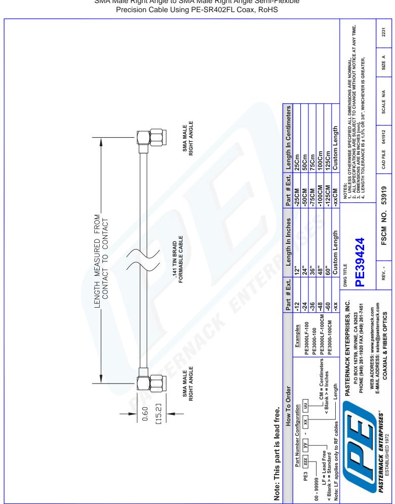
PE39424 CAD Drawing SMA Male Right Angle to SMA Male Right Angle Semi-Flexible
