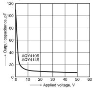
12-(2). Output capacitance vs. applied voltage characteristics
