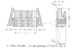
$L = (No. of poles - 1) \times pin spacing + 5 mm + 1.5 mm$  $L = (No. of poles - 1) \times pin spacing + 5 mm + 1.5 mm$
