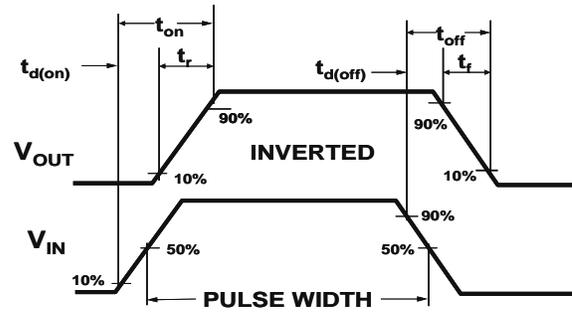
Figure 2: Switching Waveforms
