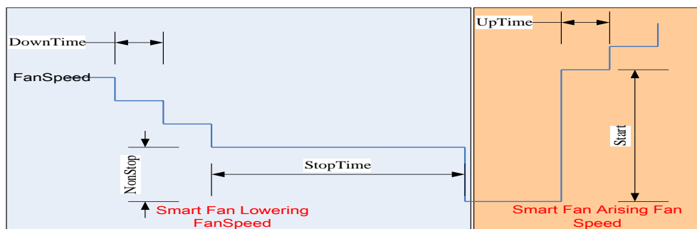
Figure 6-1 SMART FAN™ IV Control Parameters
