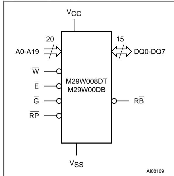
Figure 3. TSOP Connections
