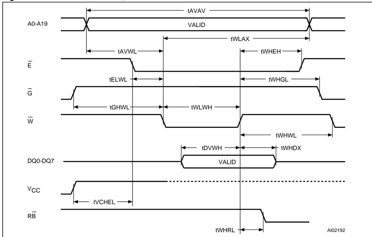
Table 12. Write AC Characteristics,  $\overline{W}$  Controlled
