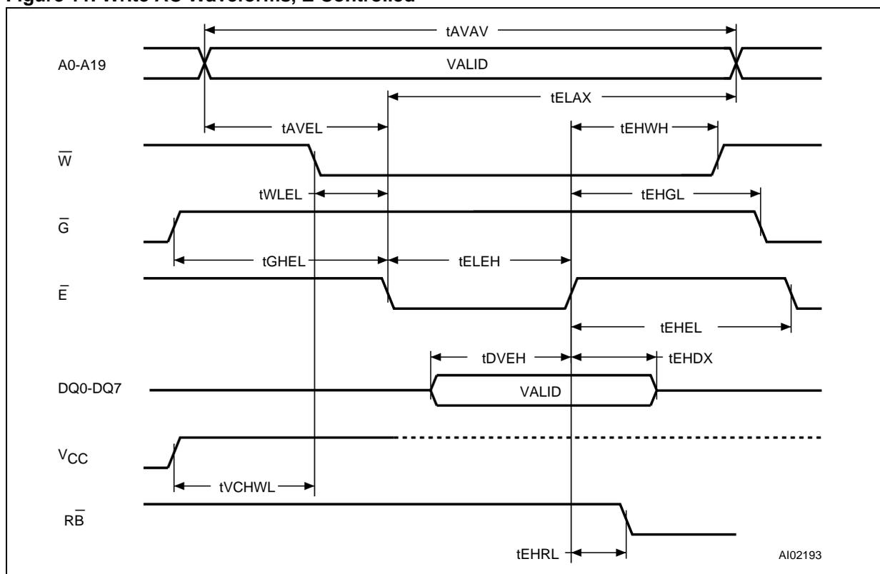
Note: 1. Address are latched on the falling edge of  $\overline{E}$ , Data is latched on the rising edge of  $\overline{E}$ .
