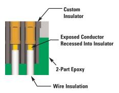
Cinch's unique plug insulators are designed to provide increased electrical protection between contact cavities preventing any potential shorts due to exposed wire or epoxy voids. Comprised of PEEK material these connectors offer superior performance and long life in severe environments.
