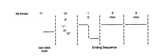
The Mini Code Violation (MCV) pattern is a bit sequence containing no mid-bit time level transition in either of its bit cells. It is a unique code that violates the encoding rules and indicates the end of valid transmit data.
