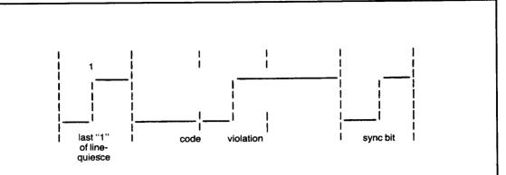
The Code Violation pattern is a bit sequence containing no mid-bit time level transition in two of its three bit cells. It is a unique pattern that violates the encoding rules and indicates the start of valid data.
