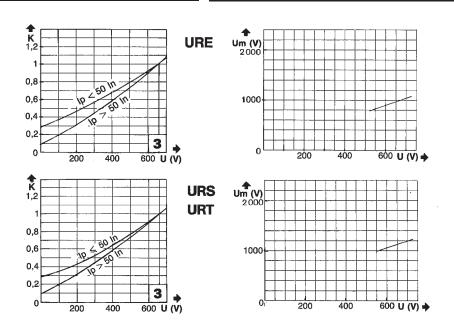
Correction Factor to determine the clearing I²t value for a fuse operating below its rated voltage
