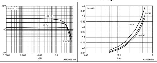
Figure 4. Base emitter saturation voltage
