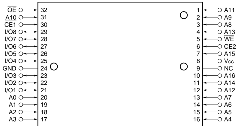
32-pin Plastic TSOP (I) (8 × 20mm) (Reverse bent) [μPD431000AGZ-KKH]
