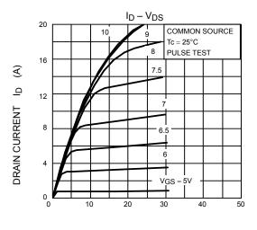
DRAIN-SOURCE VOLTAGE V<sub>DS</sub> (V)
