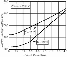
Vcontrol Dropout Voltage vs Output Current
