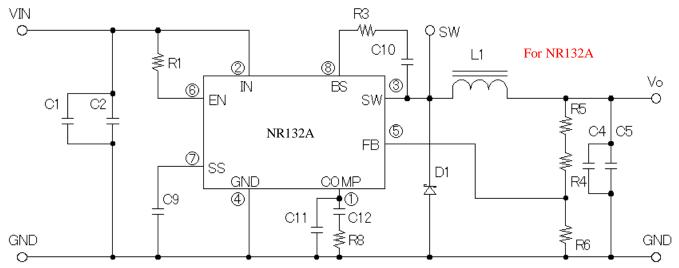
C1, C2:  $10\mu F$  / 25V, C4, C5:  $22\mu F$  / 16V, C7:  $0.1\mu F$ , C9:1800pF, C11: 220pF(Option), R1:  $510k\Omega$ , R3:  $10\Omega$ , R4: 36  $k\Omega$ , R5:  $27k\Omega$  (VO=5.0V), R6:  $12k\Omega$ , R7:510k $\Omega$ (Option), D1: SJPJ-L4, L1:  $10\mu H$
