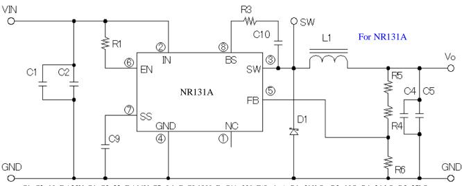
C1, C2:  $10\mu F$  / 25V, C4, C5:  $22\mu F$  / 16V, C7:  $0.1\mu F$ , C9:1800pF, C11: 220pF(Option), R1:  $510k\Omega$ , R3:  $10\Omega$ , R4:  $36~k\Omega$ , R5:  $27k\Omega$  (VO=5.0V), R6:  $12k\Omega$ , R7:510k $\Omega$ (Option), D1: SJPJ-L4, L1:  $10\mu H$
