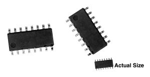
The NOMC series features a standard 14 pins and 16 pins narrow body (0.150") small outline surface mount style. It can accommodate resistor networks to your particular application requirements. The networks can be constructed with passivated nichrome (standard), or tantalum nitride (1) resistor films to optimize performance.
