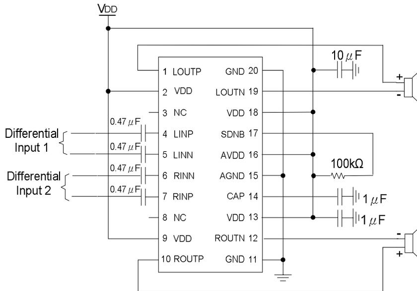
Figure.1 Differential Input With Gain =  $\frac{320k}{20k} = 16$
