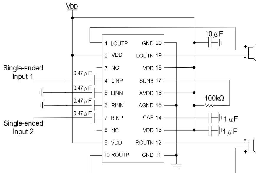
Figure.2 Single-ended Input With Gain =  $\frac{320k}{20k} = 16$
