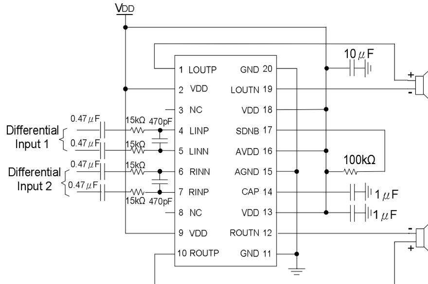
Figure.3 Differential Input With Gain =  $\frac{320k}{20k+15k} = 9.1$
