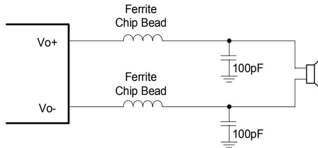
Typical Ferrite Chip Bead Filter
