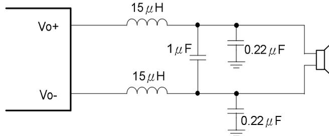
Typical LC Output Filter, Cutoff Frequency of 41 kHz,
