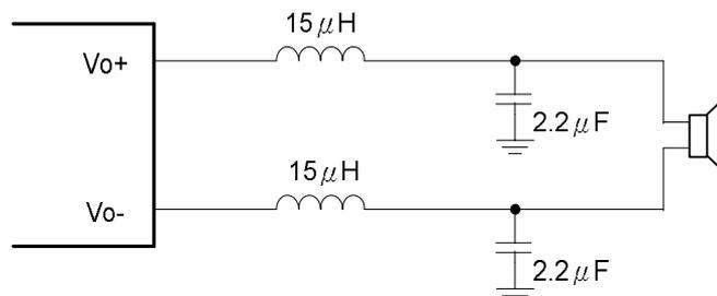
Other LC Output Filter, Speaker Impedance=3Ω & 4Ω
