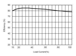
Efficiency vs Output Load (Single Output)
