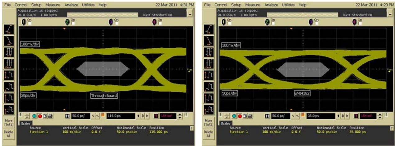
Figure 10. EMI4182MU Measured Eye Diagram @ 3.4Gbps (EVB through on left, EVB with EMI4182MU on right)
