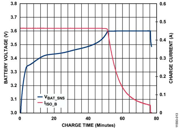
Figure 10. Charge Profile,  $ILIM[3:0] = 0110$  (Binary) = 500 mA, LiFePO<sub>4</sub>, Battery Capacity = 500 mAh
