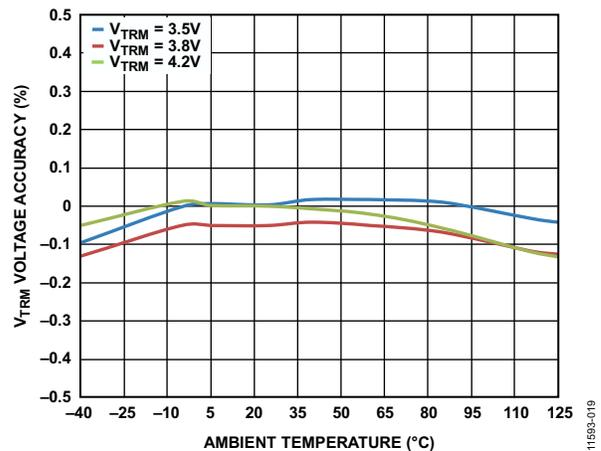
Figure 16. Termination ( $V_{TRM}$ ) Voltage Accuracy vs. Ambient Temperature
