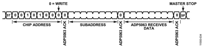
Figure 31. I<sup>2</sup>C Single Register Write Sequence
