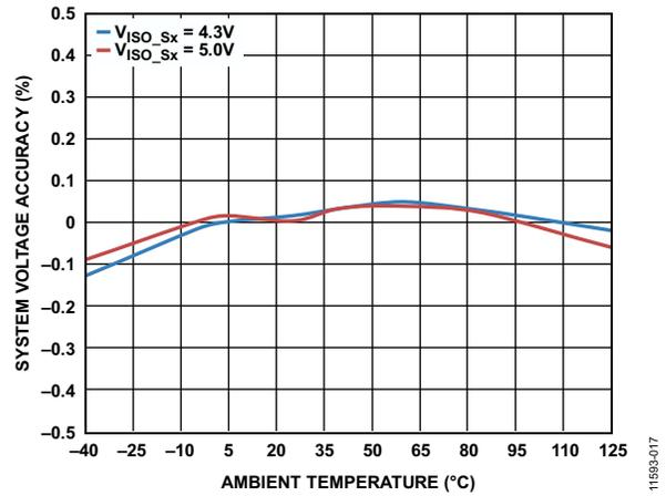
Figure 14. System Voltage Accuracy vs. Ambient Temperature, Trickle Charge Mode,  $V_{ISO\_Sx} = 4.3\text{ V}$  and  $V_{VINx} = 5.0\text{ V}$ , or  $V_{ISO\_Sx} = 5.0\text{ V}$  and  $V_{VINx} = 6.0\text{ V}$
