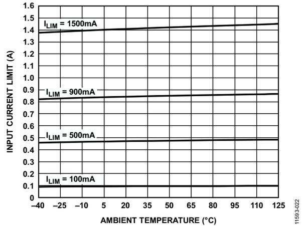
Figure 19. Input Current Limit vs. Ambient Temperature
