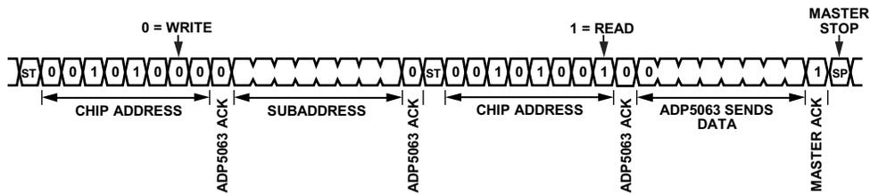
Figure 33. I<sup>2</sup>C Single Register Read Sequence
