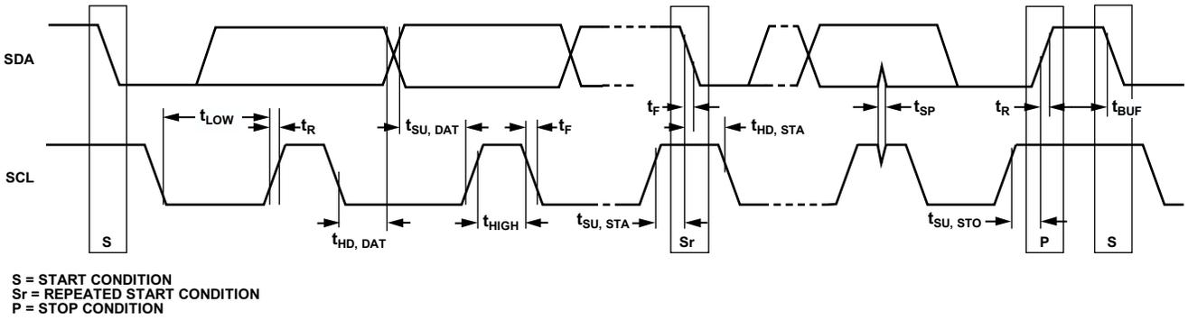
Figure 2. I<sup>2</sup>C Timing Diagram
