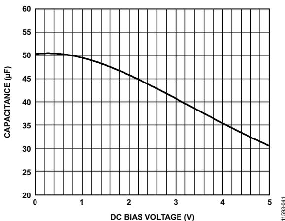
Figure 35. Murata GRM31CR61A226KE19 Capacitance vs. Bias Voltage
