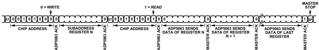
Figure 34. I<sup>2</sup>C Multiple Register Read Sequence
