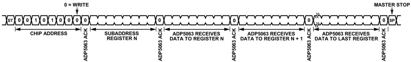
Figure 32. I<sup>2</sup>C Multiple Register Write Sequence
