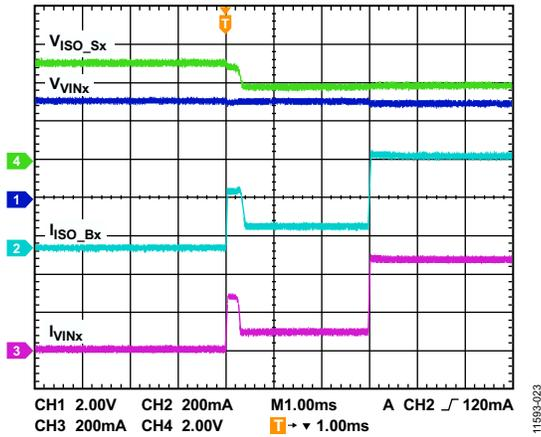
Figure 20. Charging Startup,  $V_{INx} = 5.0V$ ,  $ILIM[3:0] = 0110$  (Binary) = 500 mA,  $ICHG[4:0] = 01110$  (Binary) = 750 mA
