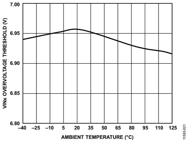
Figure 18. VINx Overvoltage Threshold vs. Ambient Temperature
