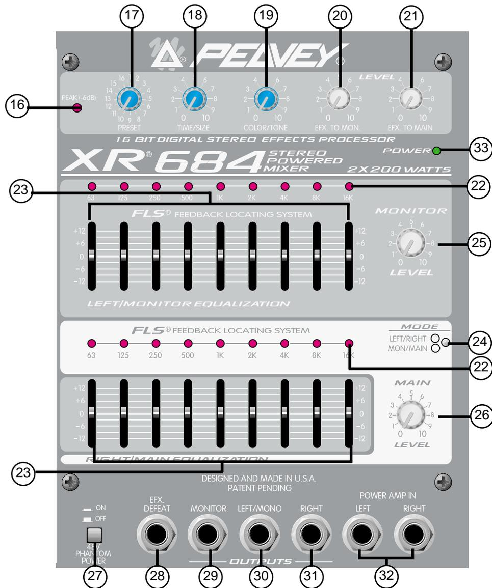
**26. MAIN LEVEL:** This is the master level control for the main mix sent to the Left/Mono and Right output jacks. This control sets the Main level going to the power amp when in Main/Monitor mode (see System Mode #24). A good starting position for this control is the center detent position (12:00).
