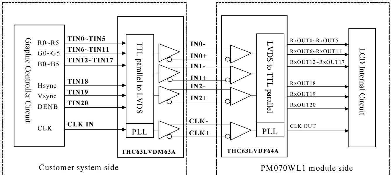
Recommended Transmitter (THC63LVDM63A Thine) to PM070WL1 interface Assignment:
