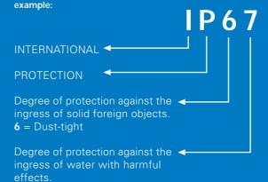
**7** = Protection against the effects of temporary immersion in water (1m submersion for 30 minutes)
