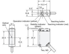
4-dia. Vinyl-insulated round cable with 4 conductors (Conductor cross section: 0.2 mm² (AWG.24), Insulator diameter: 1.1 mm), Standard length: 2 m
