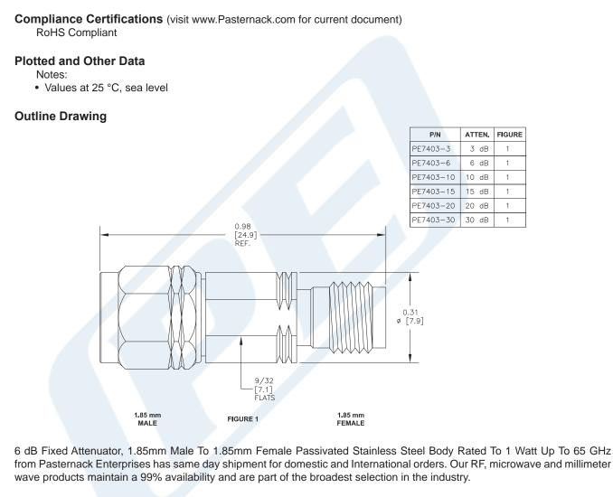
Click the following link (or enter part number in "SEARCH" on website) to obtain additional part information including price, inventory and certifications: 6 dB Fixed Attenuator, 1.85mm Male To 1.85mm Female Passivated Stainless Steel Body Rated To 1 Watt Up To 65 GHz PE7403-6
