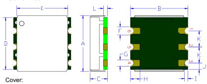
Centered on the base 304 Stainless Steel 0.010 inch (0.25mm) Electroless Nickel Plated 1 µinch (25 µm) typical
