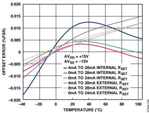
Figure 39. Offset Error vs. Temperature
