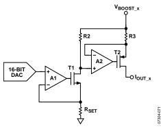
Figure 72. Voltage-to-Current Conversion Circuitry
