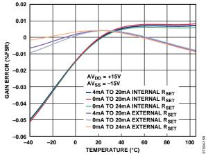
Figure 40. Gain Error vs. Temperature
