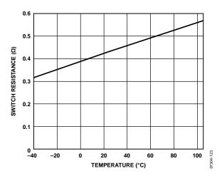
Figure 58. Switch Resistance vs. Temperature
