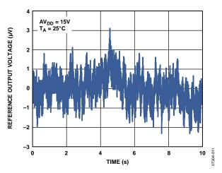
Figure 60. REFOUT Output Noise (0.1 Hz to 10 Hz Bandwidth)
