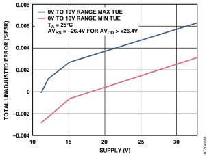
Figure 21. Total Unadjusted Error vs. AV<sub>DD</sub>/|AV<sub>SS</sub>|
