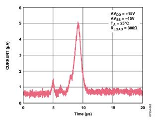
Figure 46. Output Current vs. Time on Power-Up
