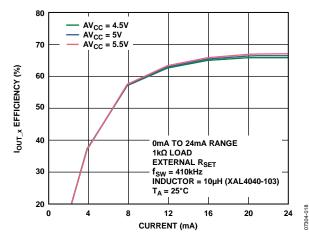
Figure 56. Output Efficiency vs. Output Current (See Figure 78)
