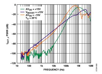
Figure 53. IOUT\_x PSRR vs. Frequency
