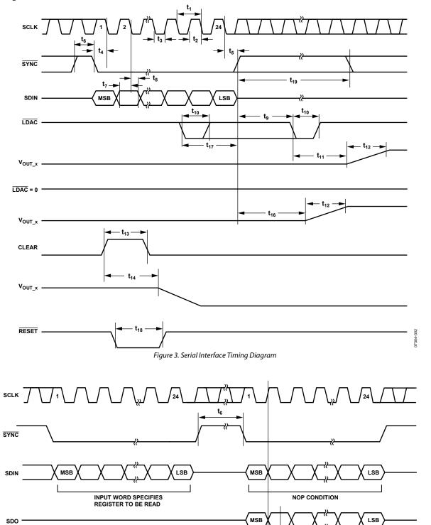
Figure 4. Readback Timing Diagram
