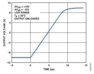
Figure 23. Full-Scale Positive Step
