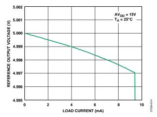
Figure 63. REFOUT vs. Load Current
