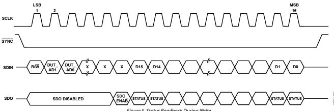
Figure 5. Status Readback During Write
