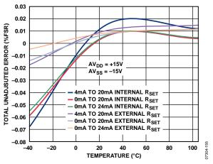
Figure 37. Total Unadjusted Error vs. Temperature
