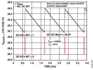
Figure 79. Operation on Reaching V<sub>MAX</sub>
