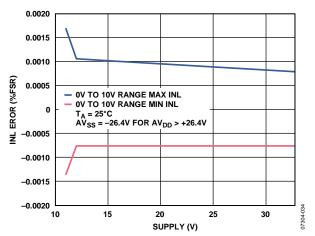
Figure 19. Integral Nonlinearity Error vs. AV<sub>DD</sub>/|AV<sub>SS</sub>|
