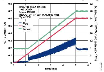
Figure 83. Alcc Current vs. Time for 24 mA Step Through 1  $k\Omega$  Load with Slew Rate Control
