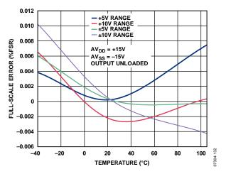
Figure 14. Full-Scale Error vs. Temperature
