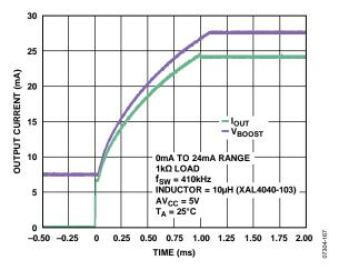
Figure 48. Output Current and V<sub>BOOST\_x</sub> Settling with DC-to-DC Converter (See Figure 78)
