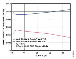
Figure 44. Total Unadjusted Error vs. AV<sub>DD</sub>, External R<sub>SET</sub>
