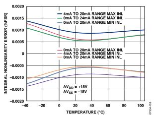
Figure 35. Integral Nonlinearity vs. Temperature, External RSET
