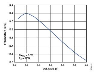
Figure 69. Internal Oscillator Frequency vs. DVcc Supply Voltage
