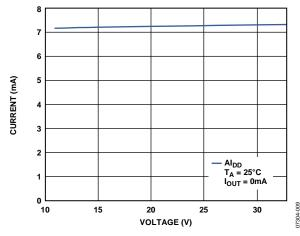
Figure 67. Al<sub>DD</sub> vs. AV<sub>DD</sub>
