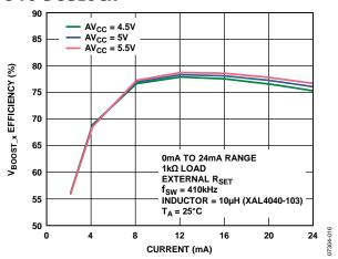
Figure 54. Efficiency at V<sub>BOOST\_x</sub> vs. Output Current (See Figure 78)
