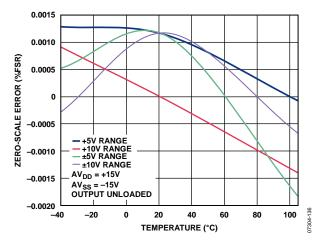
Figure 18. Zero-Scale Error vs. Temperature
