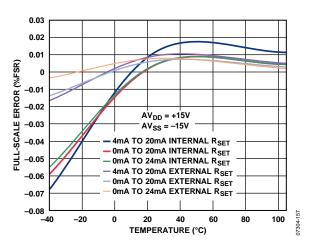
Figure 38. Full-Scale Error vs. Temperature
