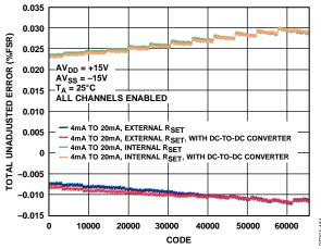
Figure 33. Total Unadjusted Error vs. Code
