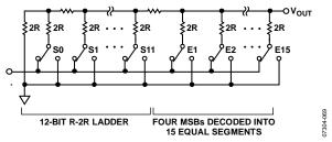
Figure 70. DAC Ladder Structure
