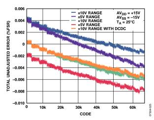
Figure 10. Total Unadjusted Error vs. DAC Code
