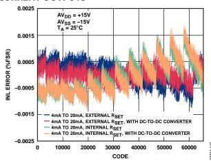
Figure 31. Integral Nonlinearity vs. Code
