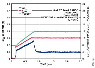
Figure 82. Alcc Current vs. Time for 24 mA Step Through 500  $\Omega$  Load with External 51 k $\Omega$  Compensation Resistor
