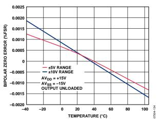
Figure 16. Bipolar Zero Error vs. Temperature
