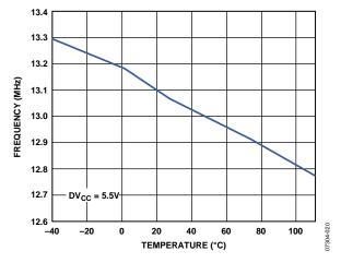
Figure 68. Internal Oscillator Frequency vs. Temperature
