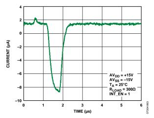
Figure 47. Output Current vs. Time on Output Enable
