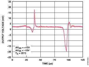
Figure 28.  $V_{OUT_{-x}}$  vs. Time on Power-Up
