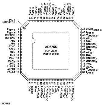
1. THIS EXPOSED PADDLE SHOULD BE CONNECTED TO THE POTENTIALOF THE AV<sub>SS</sub> PIN, OR, ALTERNATIVELY, IT CAN BE LEFT ELECTRICALLY UNCONNECTED. IT IS RECOMMENDED THAT THE PADDLE BE THERMALLY CONNECTED TO A COPPER PLANE FOR ENHANCED THERMAL PERFORMANCE.
