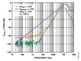
Figure 30.  $V_{OUT_x}$  PSRR vs. Frequency
