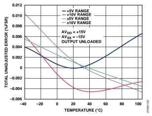
Figure 13. Total Unadjusted Error vs. Temperature
