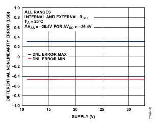
Figure 43. Differential Nonlinearity Error vs. AVDD
