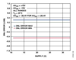
Figure 20. Differential Nonlinearity Error vs. AVDD/|AVss|
