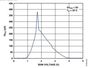
Figure 65. Dlcc vs. Logic Input Voltage
