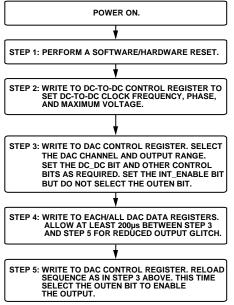
Figure 74. Programming Sequence for Enabling the Output Correctly
