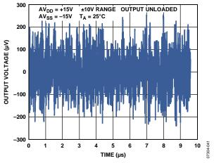
Figure 27. Peak-to-Peak Noise (100 kHz Bandwidth)
