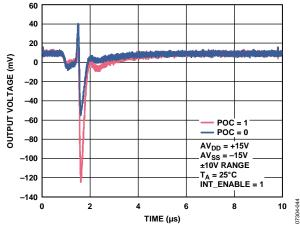
Figure 29. V<sub>OUT\_x</sub> vs. Time on Output Enable
