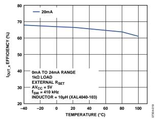
Figure 57. Output Efficiency vs. Temperature (See Figure 78)
