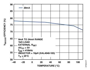
Figure 55. Efficiency at  $V_{BOOST\_x}$  vs. Temperature (See Figure 78)
