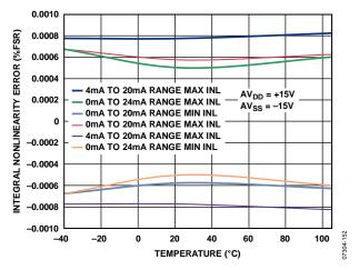
Figure 34. Integral Nonlinearity vs. Temperature, Internal RSET
