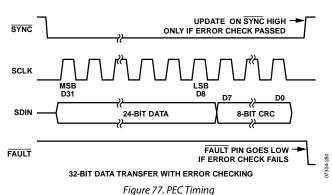
The PEC can be used for both transmit and receive of data packets. If status readback during a write is enabled, the PEC values returned during the status readback during a write
