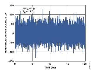
Figure 61. REFOUT Output Noise (100 kHz Bandwidth)
