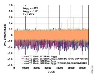
Figure 32. Differential Nonlinearity vs. Code
