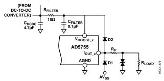
Figure 84. Output Transient Voltage Protection
