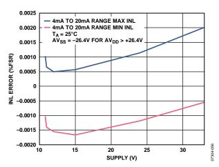
Figure 41. Integral Nonlinearity Error vs. AV<sub>DD</sub>/|AV<sub>SS</sub>|, Over Supply, External R<sub>SET</sub>
