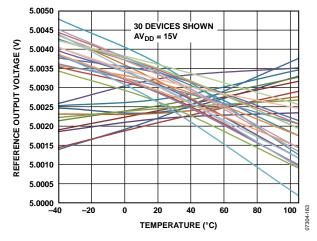
Figure 62. REFOUT vs. Temperature (When the AD5755 is soldered onto a PCB, the reference shifts due to thermal shock on the package. The average output voltage shift is -4 mV. Measurement of these parts after seven days shows that the outputs typically shift back 2 mV toward their initial values. This second shift is due to the relaxation of stress incurred during soldering.)
