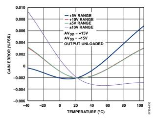
Figure 17. Gain Error vs. Temperature
