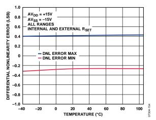
Figure 36. Differential Nonlinearity vs. Temperature
