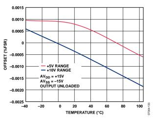
Figure 15. Offset Error vs. Temperature
