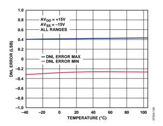
Figure 12. Differential Nonlinearity Error vs. Temperature
