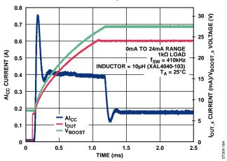
Figure 80. Al $_{CC}$  Current vs. Time for 24 mA Step Through 1 k $\Omega$  Load with Internal Compensation Resistor
