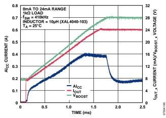
Figure 81. Alcc Current vs. Time for 24 mA Step Through 1  $k\Omega$  Load with External 51  $k\Omega$  Compensation Resistor
