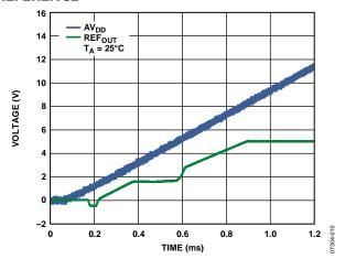
Figure 59. REFOUT Turn-On Transient
