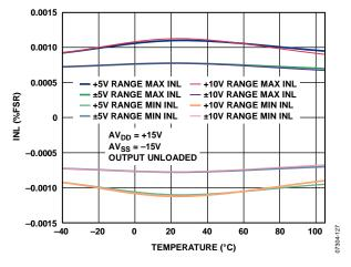
Figure 11. Integral Nonlinearity Error vs. Temperature
