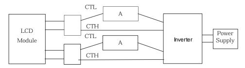
\*2)Lamp frequency of inverter may produce interference with horizontal synchronous frequency, and this may cause horizontal beat on the display. Therefore, please adjust lamp frequency, and keep inverter as far from module as possible or use electronic shielding between inverter and module to avoid the interference.
