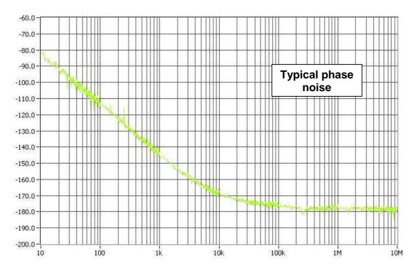
Nota: Typical phase noise of one oscillator measured with the new DCNTS from Aeroflex
