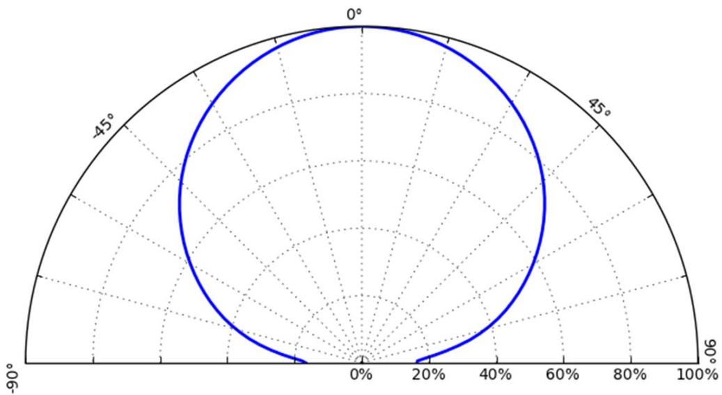
Figure 10. Typical representative polar radiation pattern for LIQ0-xyy00000zzz0.
