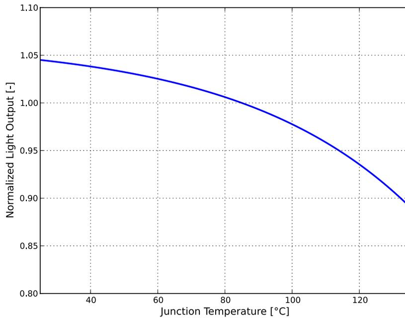
Figure 6. Relative light output vs. junction temperature, LIQ0-xyy00000zzz0.
