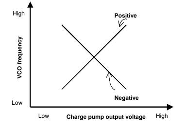
Fig. 11 Charge Pump Output Polarity
