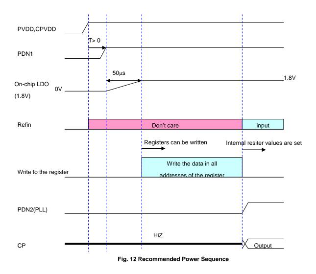
Note 1) The initial register values are not defined. Therefore, even after [PDN1] is set to "High", each bit value remains undefined. In order to set all register values, it is required to write the data in all addresses of the register.
