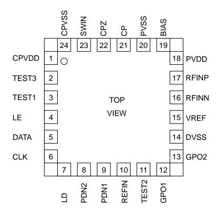
Fig. 2 Package Pin Layout
