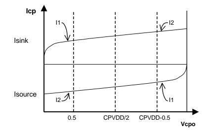
Fig. 4 Charge Pump Characteristics - Voltage (Vcpo) vs. Current (lcp)
