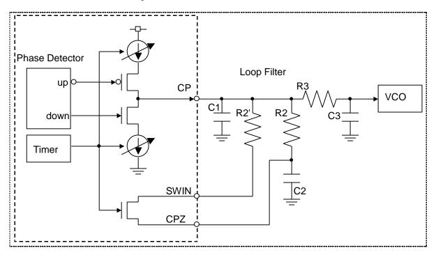
Fig. 5 Loop Filter Schematic
