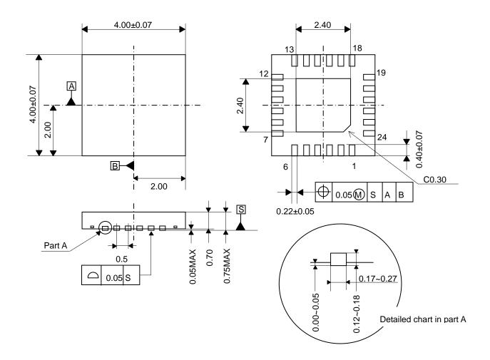
Fig. 16 Package Outer Dimensions
