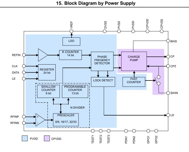
Fig. 15 Power Supply Block Diagram
