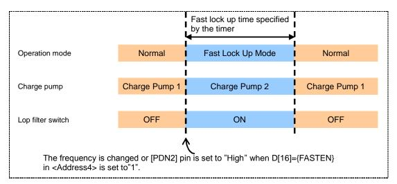
Fig. 6 Timing Chart for Fast Lock Up Mode
