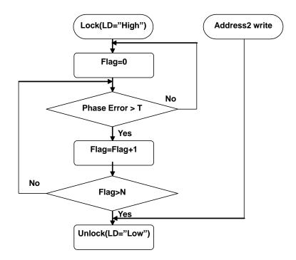
Fig. 10 Transition Flow Chart: Lock State to Unlock State
