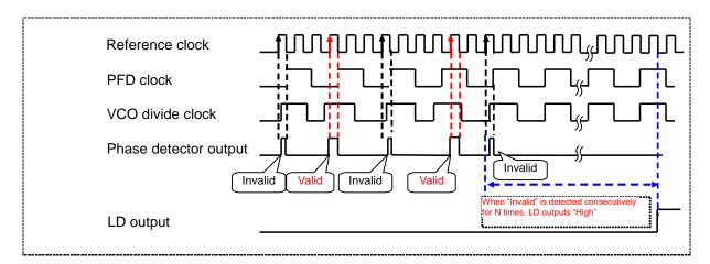
Fig. 8 Digital Lock Detect Operations
