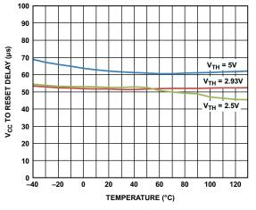
Figure 9.  $V_{CC}$  to Reset Delay vs. Temperature
