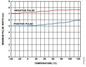
Figure 15. Watchdog Input Minimum Pulse Width vs. Temperature
