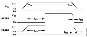
Figure 20. Reset Timing Diagram
