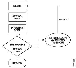
Figure 23. Watchdog Flow Diagram
