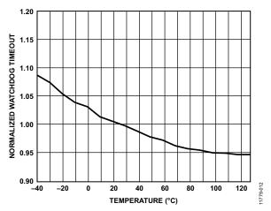
Figure 12. Normalized Watchdog Timeout vs. Temperature
