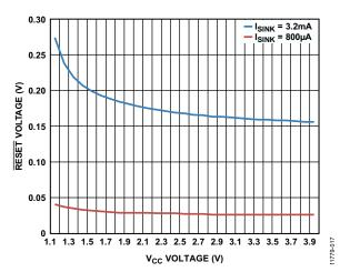
Figure 17.  $\overline{RESET}$  Push-Pull  $V_{OL}$  Voltage vs.  $V_{CC}$  Voltage ( $V_{TH} = 4 V$ )
