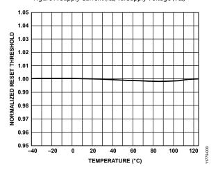
Figure 8. Normalized Reset Threshold vs. Temperature
