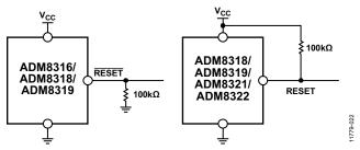
Figure 22. Ensuring Reset Valid to  $V_{CC} = 0 V$
