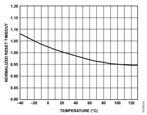
Figure 11. Normalized Reset Timeout vs. Temperature
