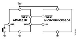
Figure 24. Typical Application Circuit
