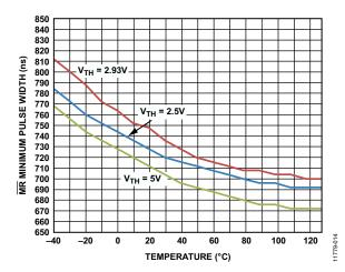
Figure 14. Manual Reset (MR) Minimum Pulse Width vs. Temperature
