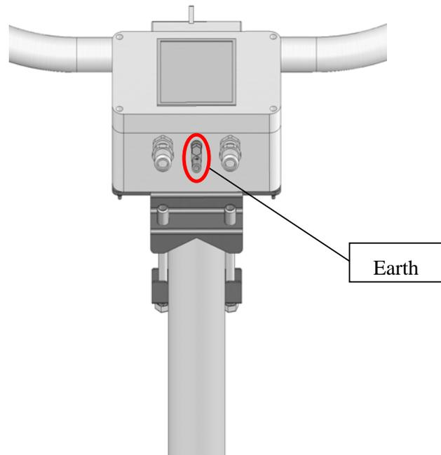
The CS120 must be properly grounded by taking a ground wire with a minimum cross sectional area of  $6 \text{ mm}^2$  and maximum length of 5 m from the brass grounding lug in the lower face of the electronics enclosure to an adequate grounding point. The pole and foundations of a pole mounted installation will provide some basic lightning protection and protection against radio frequency interference and should also be correctly grounded.
