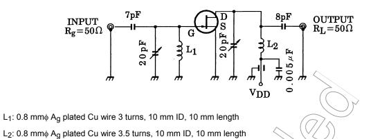
Figure 1 100 MHz Gps NF Test Circuit
